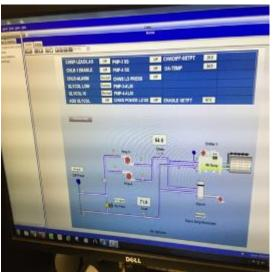
Image 6: AAON RTU & Metasys Chilled Water Control System
