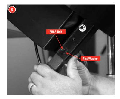
Place a ¼" Flat Washer (31) over the end of each of the two Bolts just previously place through the Bullet Feed Hopper and Square Tubing Mounting Bracket.
