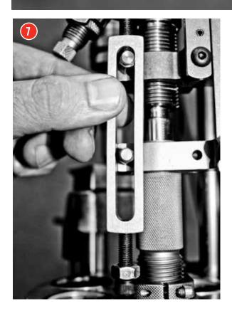
Place an empty, primed case into the station of the shell plate that will rotate to the powder measure. Raise the ram which will cycle the powder measure to the top of its stroke. Thread the bottom cap screw in until the threaded end bottoms out on the lower hex spring mount.
