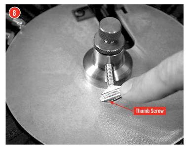
**g** Loosen Lock Nut (7) on the Adjustment Screw (6).
