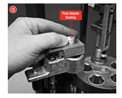
Place the Pivot Adapter on top of the pivot for rifle cases. **Refer to page 45 for proper Pivot Adapter.**
