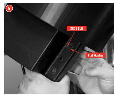
6 Place a ¼-20 X 2 SHCS Bolt (30) with one ¼" Flat Washer (31) thru the bottom hole of the Bullet Feed Hopper and the Square Tubing Mounting Bracket.
