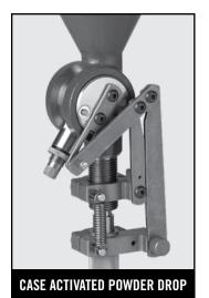
The Case Activated Powder Drop has been engineered with quick change-overs in mind. The retainer spring offers smooth function and the powder drop only dispenses a powder charge when a case is present. Works with the L-N-L AP or other progressive presses that use 7/8" x 14 threads.
