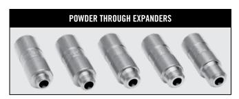
Powder Through Expanders (PTX) are designed to work in conjunction with the Case Activated Powder Drop, these new Expanders eliminate the need for a separate case mouth expander die on the L-N-L AP progressive press (Hornady suggests you fill that station with the powder cop die, so you can ensure that each case is properly charged with powder.)
