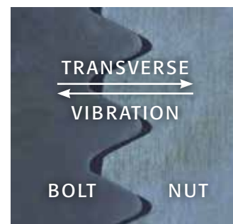
Thread Flanks can slide. Nut can move relative to bolt.
