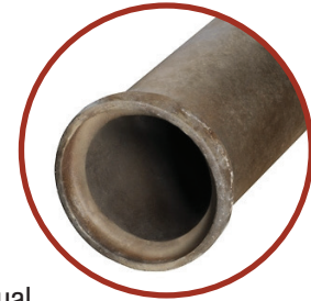
120-year-old pipe recently replaced to upsize the service line.
