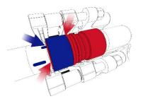
Figure 31: Lokring Fitting Installation Using the Guide-Rod Tools
