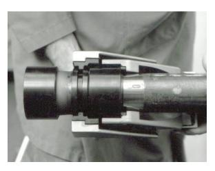
Figure 39: Driver Driven to Contact Tool Flange
