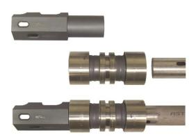
Figure 36: Using the Gauge as a Stop
