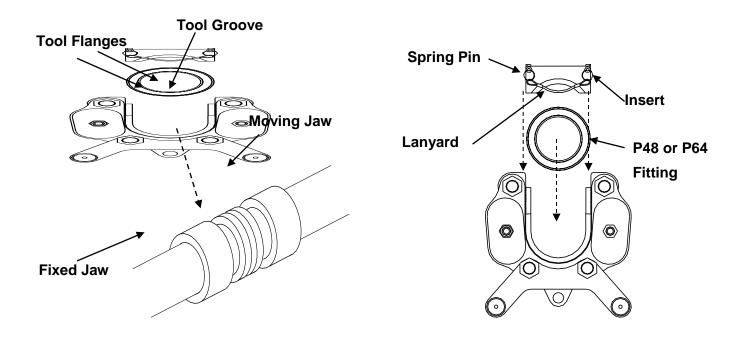
Figure 32: 3- and 4-Inch Fitting Assembly
