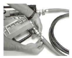
Figure 26: Installing Jaw Insert and Connecting Tool to Pump
