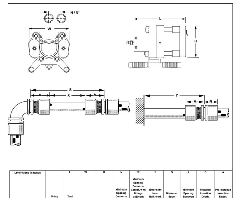
Note: Spool lengths are for reverse operation, except where noted. Spool lengths may be decreased slightly if one fitting end can be pulled up prior to positioning the second end and the reverse position of the tool is used for the installation.
