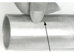
Figure 13: Longitudinal Scratches
