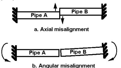
Figure 2: Examples of Pipe/Tube End Misalignment
