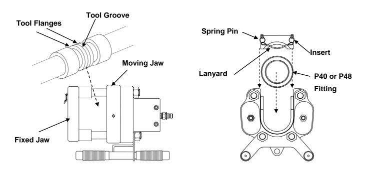
Figure 43: 2 1/2- and 3-Inch Fitting Assembly
