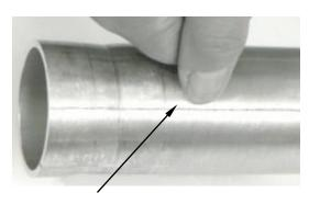
Figure 15: Weld Seam Suck-Back
