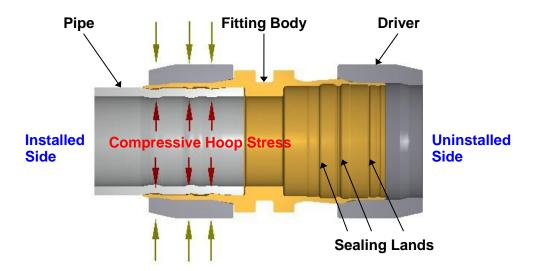
Figure 1: Installed and Sectioned Pipe Fitting
