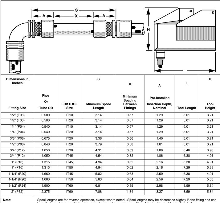
be pulled up prior to positioning the second end and the reverse position of the tool is used for the installation.
