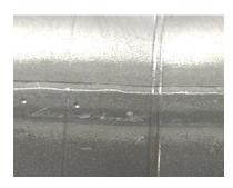
Figure 17: Seam Misalignment
