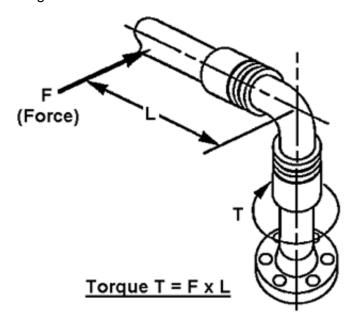
Figure 3: Application of Torque Loads During Fit-Up
