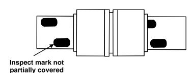
Figure 47: Incomplete Installation
