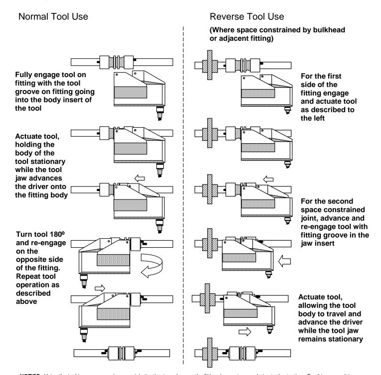
**NOTICE:** Using the tool in reverse requires special attention to make sure the fitting does not move during tool actuation. For this reason it is recommended that where possible the first joint is pulled up in normal fashion to lock the fitting in place.
