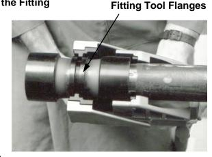
Figure 38: Tool Engaged on Fitting
