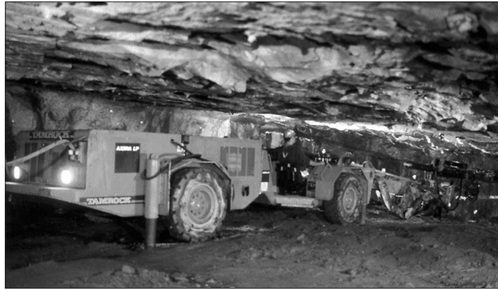
Figure 5. Tamrock Axera LP face drill rig operating in underground BIC mine
