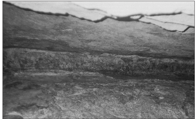
Figure 11. Mined stope after water jet cleaning
