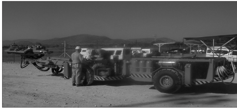
Figure 7. Long hole drilling rig on the surface
