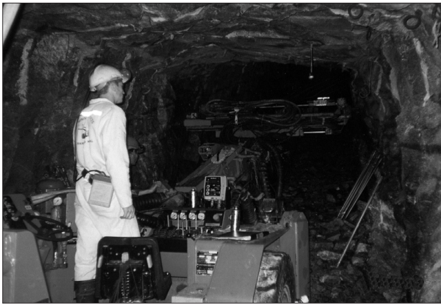
Figure 8. Long hole drilling operating in drilling raise
