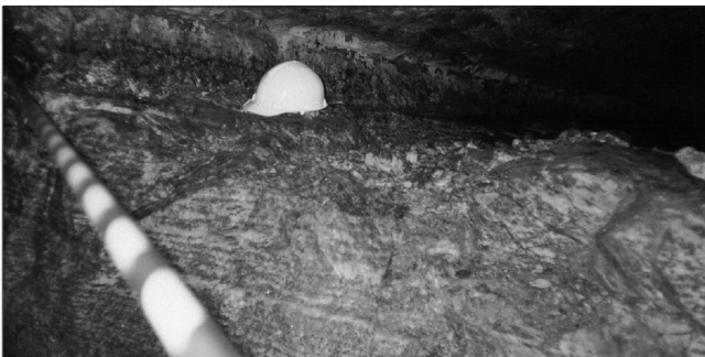
Figure 10. Blasted stopes showing hole accuracy and narrow stope
