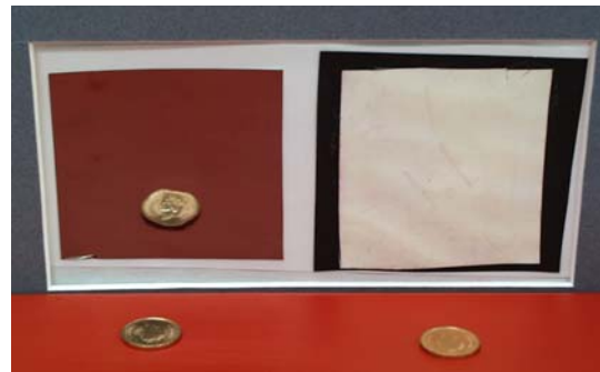
Fig.3. Optical images of Ag/Teflon samples before (left) and after (right) treatment with the texturing process. Coins are placed in front of the samples to demonstrate the total loss of reflectance in the treated sample.
