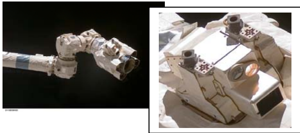
Fig.4. Image of a portion of the Canadarm2 with the camera and light on the tip of the Canadarm2. The insert shows the camera in greater details. The areas with Silver-coated Teflon are on the central part of the camera. The two side areas are blanketed.
