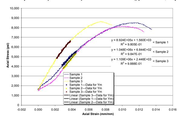
Some of the variation in the Young's modulus data could be attributed to settling of the cement slurry. The samples were cured in molds that were 10 in. long, and the individual 3-in. samples were then cut from the 10-in. specimens. For future testing, to avoid potential slurry settling, the slurry will be preconditioned for 20 minutes in an atmospheric consistometer and then poured into individual, shorter molds so only one individual test sample will come from each mold.
