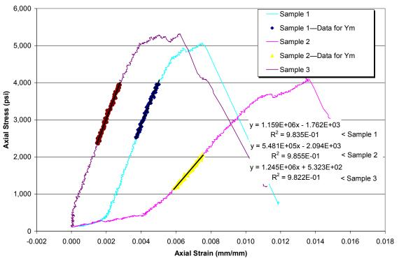
Figure 7—Young's modulus testing for samples cured in an unconfined condition and then temperature –cycled for five days and tested at a confining pressure of 1,500 psi
