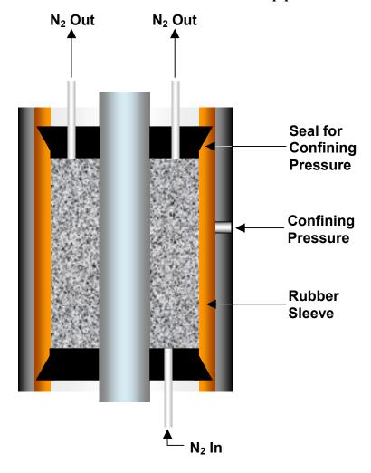
Figure 13—Cross section of annular seal model for pipe-in-soft configuration
