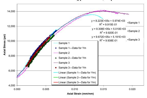
Figure 5—Young's modulus testing for samples cured in a confined condition and tested at zero confining pressure
