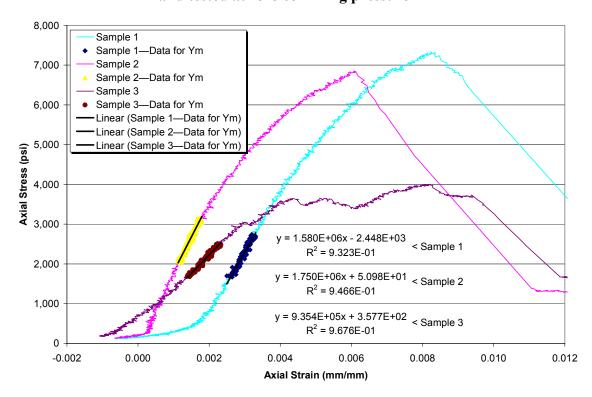
Tests were also conducted to determine the effect that temperature cycling has on Young's modulus. The temperature cycling procedure was designed to simulate temperature conditions that might be encountered during production of a well. The samples are first cured for 14 days in a 45°F water bath at atmospheric pressure. They are then subjected to five days of temperature cycling. During each of these five days of temperature cycling, the cured samples are cycled as follows.
