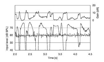
**Figure 2.** Segment of time course of signal levels in measurement 1 at Input SNR = +10 dB and corresponding gain values applied by the hearing aid. Level and gain values are derived from true root mean square for each 10 msec. Lower two curves: input signals speech S1 (thick line) and noise N1 (thin line). Upper curve: hearing aid gain.
