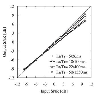
**Figure 5.** Results of measurements 7–10: signal-to-noise ratio (SNR) for single-channel compression; compression ratio 2:1; compression time constants (attack/release [Ta/Tr]) = 5/26 msec, 10/100 msec, 22/400 msec, and 50/1550 msec; speech S1 in modulated noise N2.
