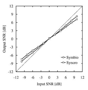
**Figure 7.** Results of measurements 13–14: signal-to-noise ratio (SNR) for single-channel very fast-acting compression, compression ratio 2:1, speech S1 in speech N3. Measured with Oticon Syncro II and Bernafon Symbio 100.
