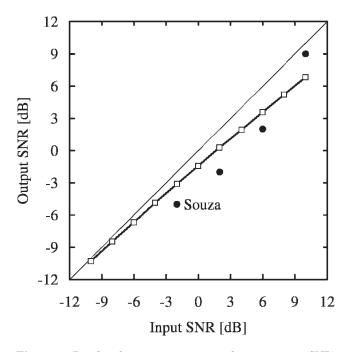
**Figure 1.** Results of measurement 1: signal-to-noise ratio (SNR) for single-channel fast-acting compression, compression ratio 2:1, speech S1 in unmodulated noise N1. Diagonal line indicates equality between Input SNR and Output SNR. Additional points ("Souza") show data for corresponding measurement from Souza et al, 2006, Table 1.
