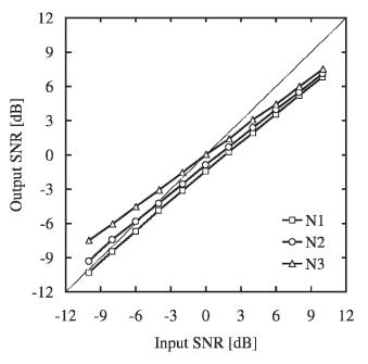
**Figure 3.** Results of measurements 1–3: signal-to-noise ratio (SNR) for single-channel fast-acting compression; compression ratio 2:1; speech S1 in unmodulated noise N1, modulated noise N2, and speech N3.
