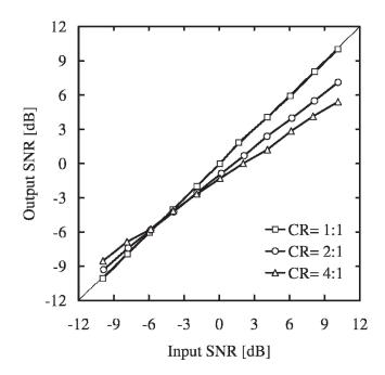
**Figure 4.** Results of measurements 4–6: signal-to-noise ratio (SNR) for single-channel fast-acting compression; compression ratios (CRs) = 1:1, 2:1, and 4:1; speech S1 in modulated noise N2.
