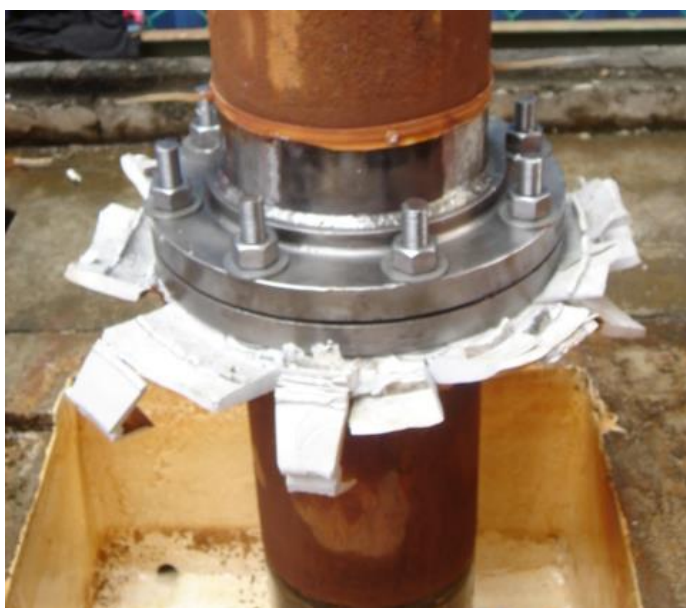
Fig 34 - Complete removal of the material shows no corrosion on substrate
