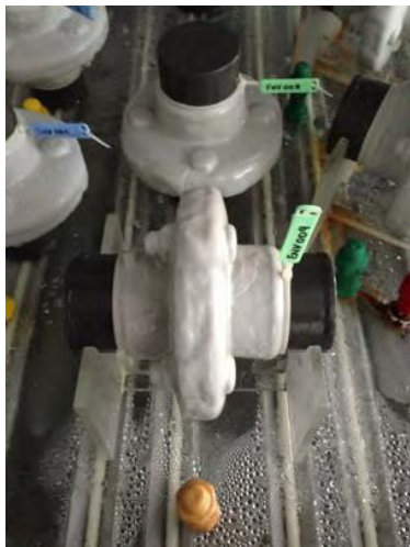
Fig 19 - Sample at 2520 hours back in hot salt fog
