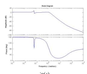
**Figure 5.2** Magnitude plot for  $\frac{\dot{\alpha}(s)}{\delta_e(s)}$  transfer function versus
