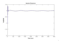
Figure 8.4 Transient response of the aircraft for  $\hat{\theta}^{c}$
