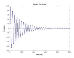
Figure 8.1 Transient response of the aircraft for  $\dot{u}$
