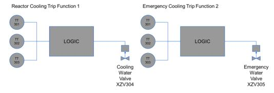
These two examples of instrumented functionality were found as separate IPLs in a LOPA assessment. Both were credited as protection against reaction runaway<sup>12</sup>. Closer inspection reveals that these apparently separate functions actually use the same set of temperature sensors. All the sensors and both valves are really part of the same function and should be considered as a single IPL with an architecture as shown in Figure 13.
