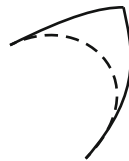
Fig. 17.9. Smoothing a corner.
