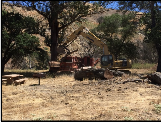
2017 photo of tub grinder and excavator chipping logs and slash
