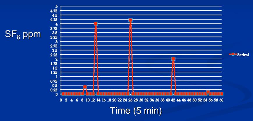
Note: periodic SF<sub>6</sub> release verified with modified smoke test.
