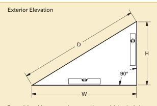
Step #4a: Measure the opening width, height and diagonal side. Based on these dimensions, louver dimensions will be corrected to obtain 90° between width and height.
