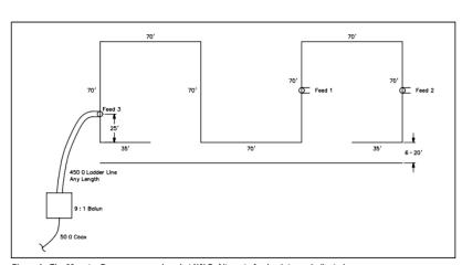
Figure 4—The 80-meter Bruce array employed at N6LF. Alternate feed points are indicated.
