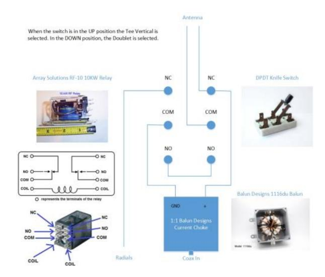
You can easily turn an inverted vee into A top hatted vertical just by using a single High power relay
