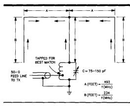
Fig 62—The bobtail curtain is an excellent low-angle radiator having broadside bidirectional characteristics. Current distribution is represented by the arrows. Dimensions A and B (in feet, for wire antennas) can be determined from the equations.
