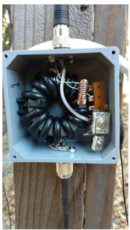
RX Phased Vertical Tuned Circuits
