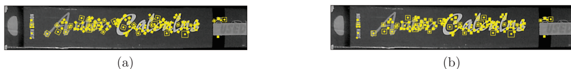
Figure 7. Segmented spine with (a) Oriented SURF keypoints and (b) Upright SURF keypoints.
