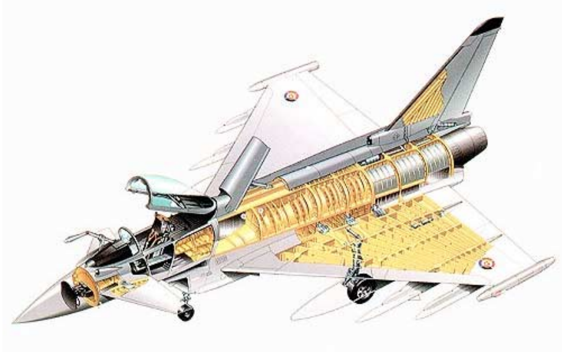
Figure 4. Cutaway view of the Eurofighter Typhoon structure.
