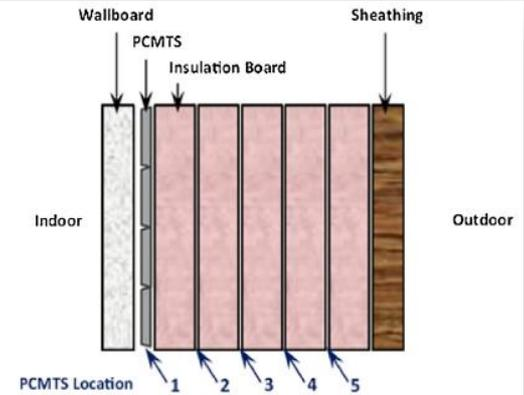
Fig. 37. Sheet of PCM thermal shield PCMTS (left) and wall section showing the PCMTS location (right) [96].
