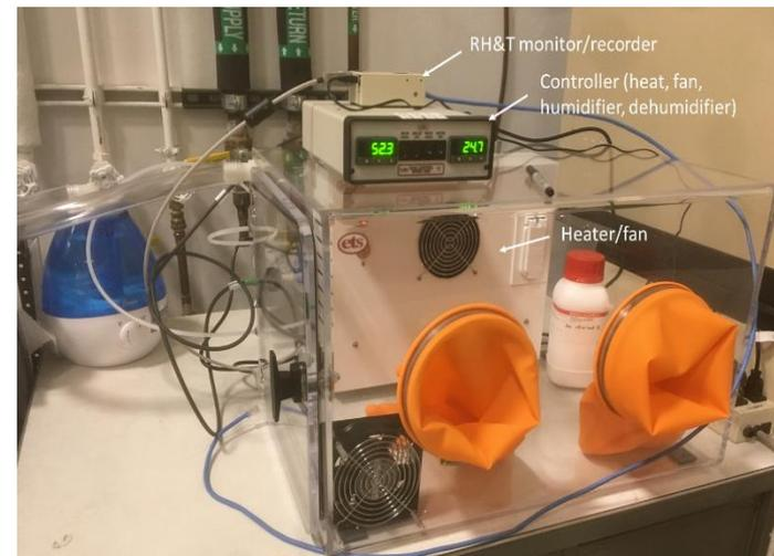
***Humidity controlled glovebox for sample transfers***
