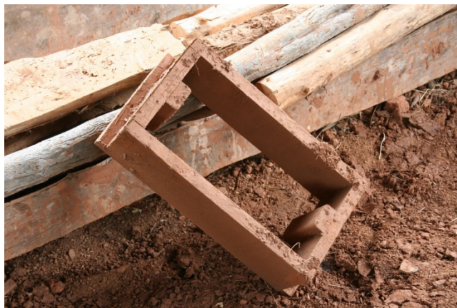
Picture 13. A mould used to shape the Adobe blocks. [18]
