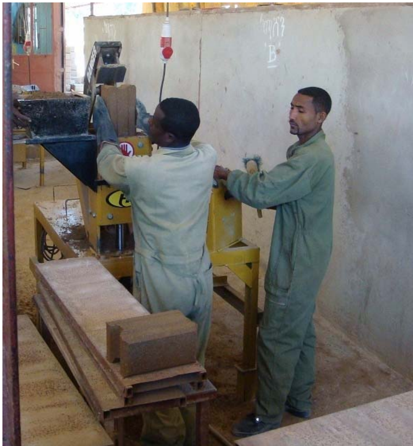
Picture 2. Hydraulic manufacturing of CSSB at Selam Technical and Vocational Centre in Addis Abeba. [5]
