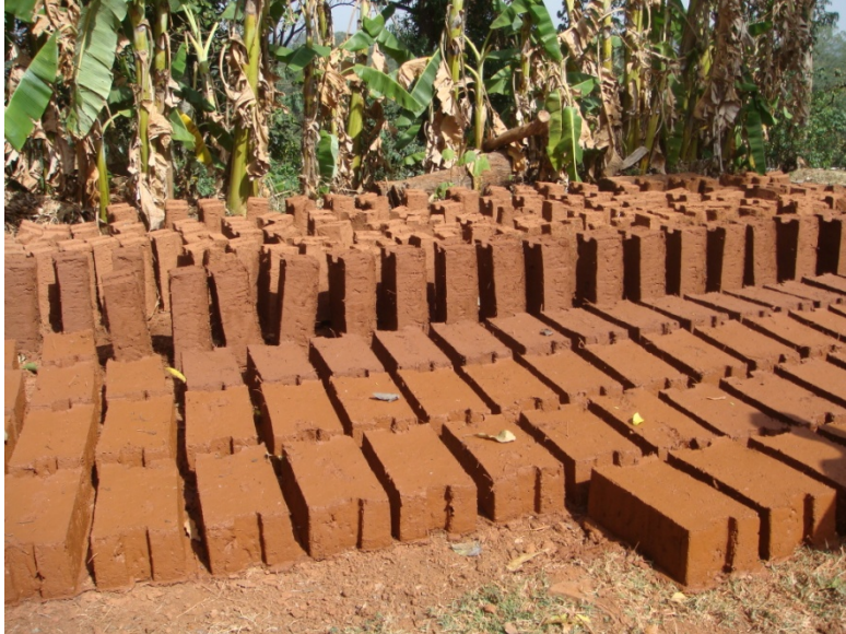
Picture 14. Recently made Adobe blocks at BTS in Challia. [5]
