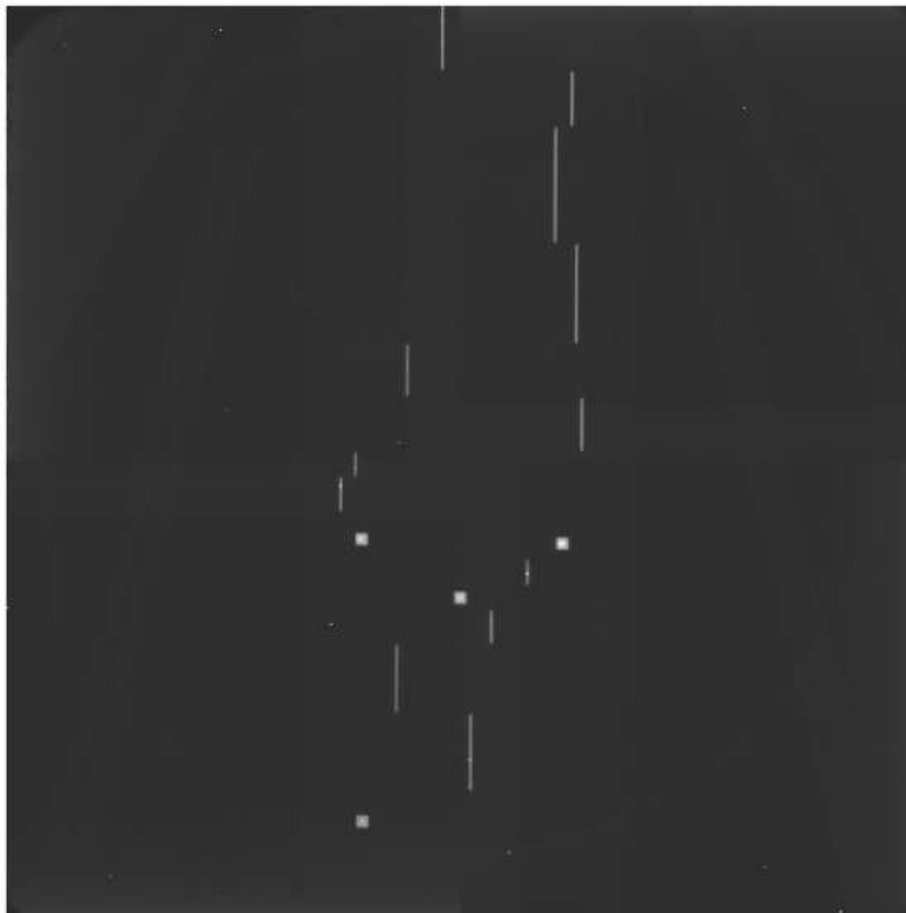
Figure 2–15. Image of a properly aligned MOS plate. The plate shown is n2071a2 ( c.f. Figure 2–14) with North up and East left. Note that all of the setup boxes contain reasonably centered stars.
