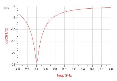
Figure 8: Input return loss of the LNA
