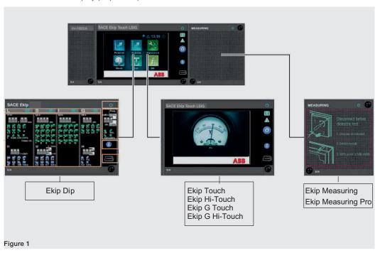
All trip units have protection and measuring functions that refer to the primary currents of the installation and are available in the following versions:
