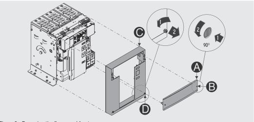
Figure 9 - Removing the flange and front cover
