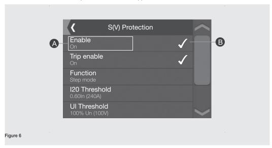
The ticks indicate that the changes are not effective. In order make a change effective, the trip unit must be programmed. To program the trip unit, you need to press the key HOME, that opens the page Programming. Alternatively, you can go up to the higher level menus until the page is displayed.
