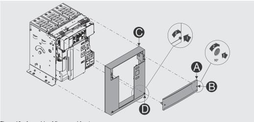
Figure 10 - Assembly of flange and front cover
