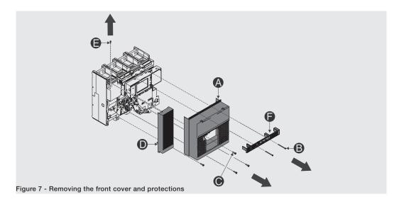
After reassembling the accessories, the parts previously dismantled must be reassembled as indicated:
