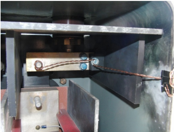
Test 15: AΦ to Case - 2-#14 - 0.35 cycles
