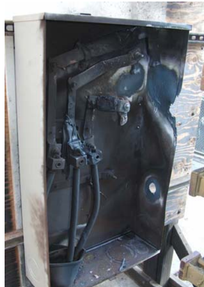
Test Specimen from Fig. 16 Post-Test
