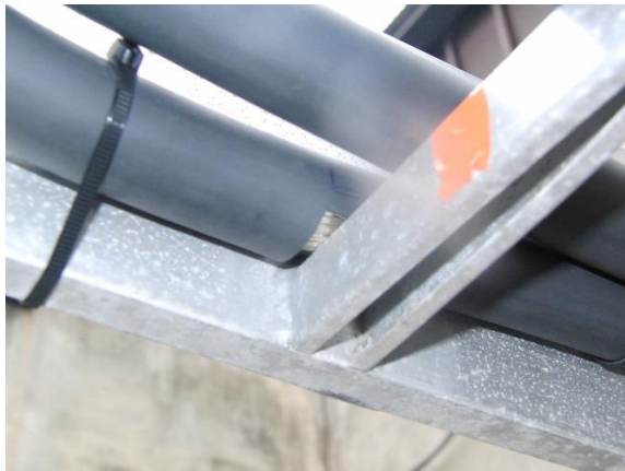
Fig. 24 Phase to ground in cable tray- 3.52 cycles
