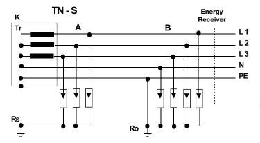
TN-S the supply network has a connection of the neutral conductor with the earthing conductor at the feeding transformer only
