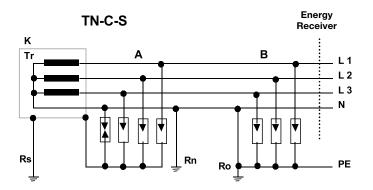
TN-C-S the neutral conductor is earthed at the transformer and in other network points
