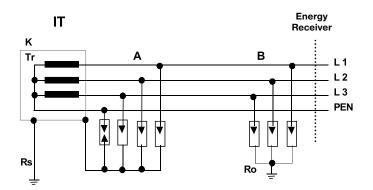
IT in this system there is no direct connection of active network parts with earth, while accessible conducting parts of installation elements are earthed
