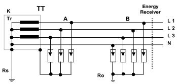
TT neutral point of transformer is earthed directly, while the receiver's installation is earthed by a separate earth electrode
