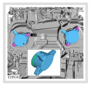
Remove the variable valve timing solenoids.
