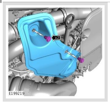
Remove the 2 retaining bolts and the Noise, Vibration and Harshness (NVH) material.
