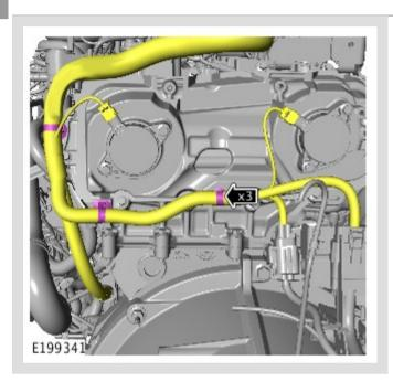
Remove the variable valve timing wiring harness from the 3 clips.
