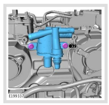
Remove the coolant separator.
