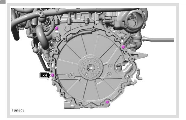
Install 2 more bolts as illustrated and tighten the 4 bolts to the final correct torque. *Torque:* **25 Nm**
