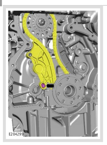
Remove the timing chain guide bolt.
