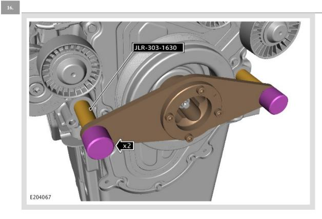
Install the special tool JLR-303-1630 to lock the crankshaft.
