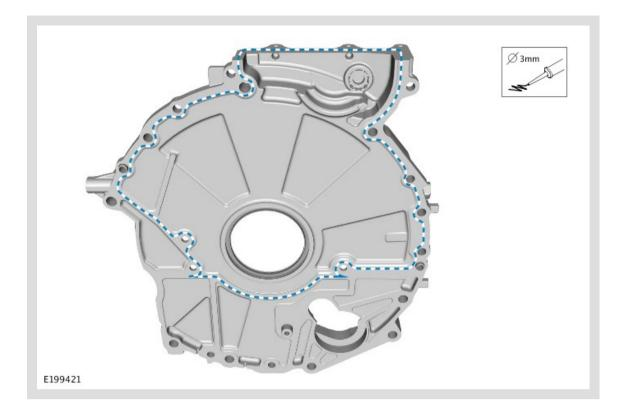
Apply a 3 mm diameter continuous bead of sealant, to the area shown. Refer to: Specifications (303-01 Engine - INGENIUM I4 2.0L Petrol, Specifications).
