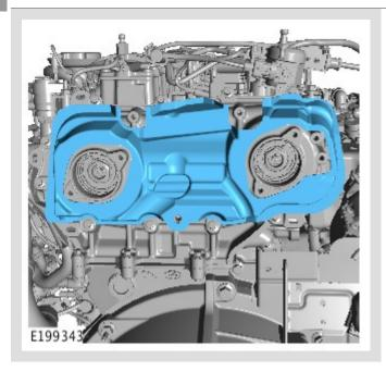
Remove the Noise, Vibration and Harshness (NVH) pad.
