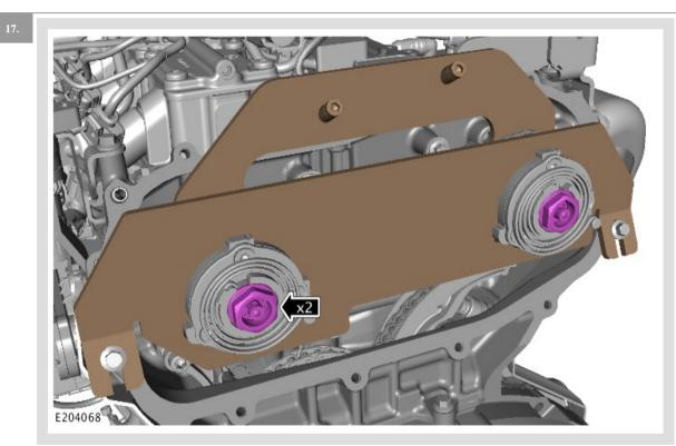
Fully tighten the VCT bolts.
