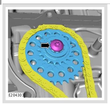
Remove the idler sprocket.
