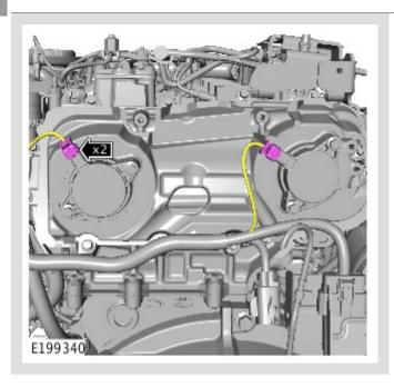
Disconnect the 2 electrical connectors from the variable valve timing solenoids.
