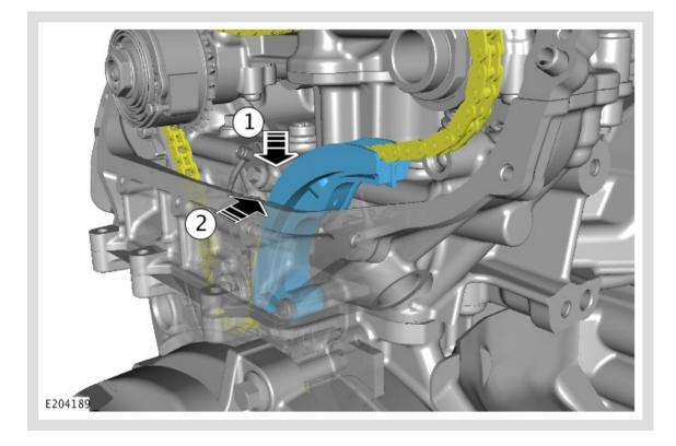
Install a new upper timing chain tensioner arm.
