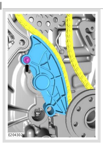
Remove the timing chain guide and bolt.
