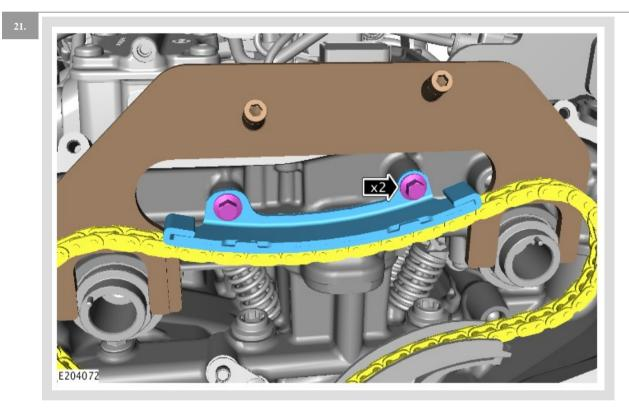
Remove the timing chain guide.
