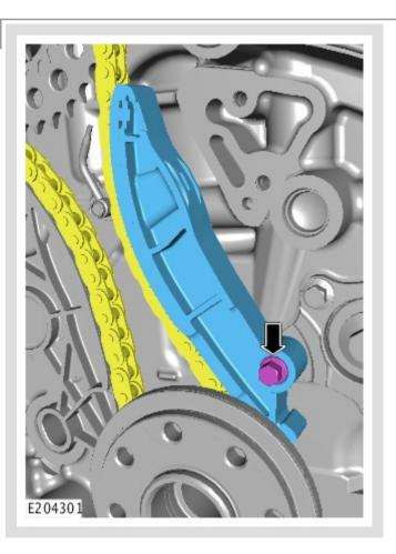
Install the timing chain tensioner guide and bolt.
