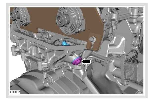
Install and tighten the new timing chain tensioner. Renew Part: Upper timing chain tensioner Quantity: 1 . Torque: **55 Nm**
