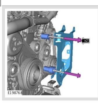
Remove the charge air radiator bracket.
