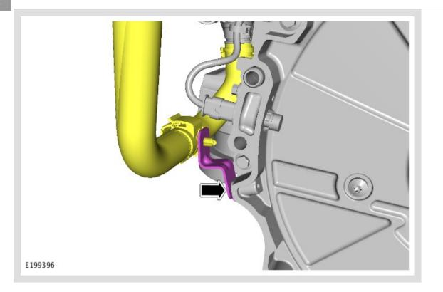
Remove the coolant pipe bracket.
