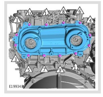
Install the upper timing cover in the sequence shown. *Torque:*
