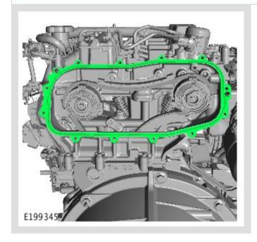
Remove the upper timing chain cover gasket.
