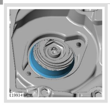
Lubricate the variable valve timing solenoid bore with clean engine oil.
