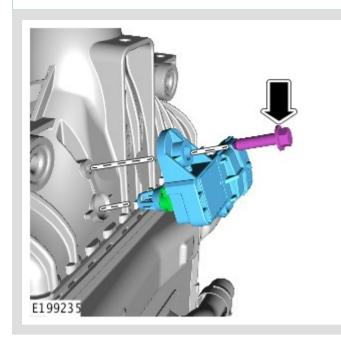
Remove the retaining bolts and the charge air cooler temperature and pressure sensor.
