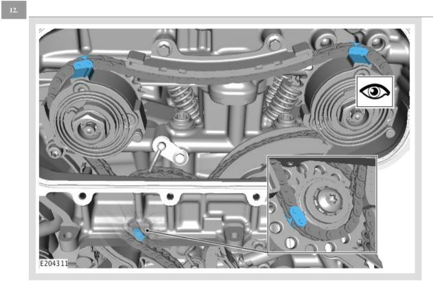
Make sure that the timing marks aligns as illustrated.
