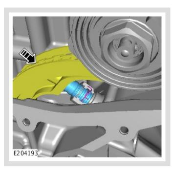
• Release the secondary timing chain tensioner piston.
