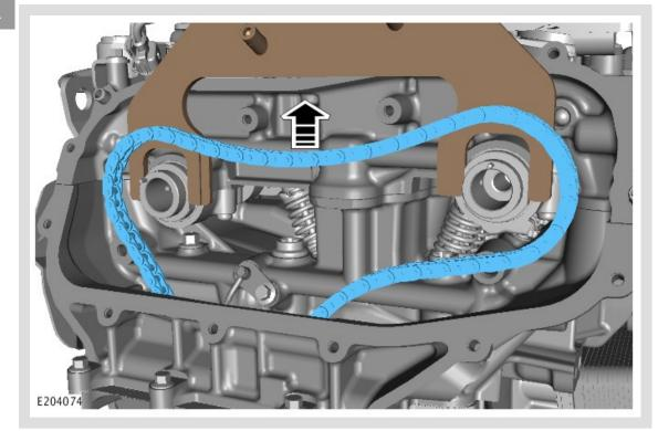
• Release the timing chain from the idler sprocket and remove.
