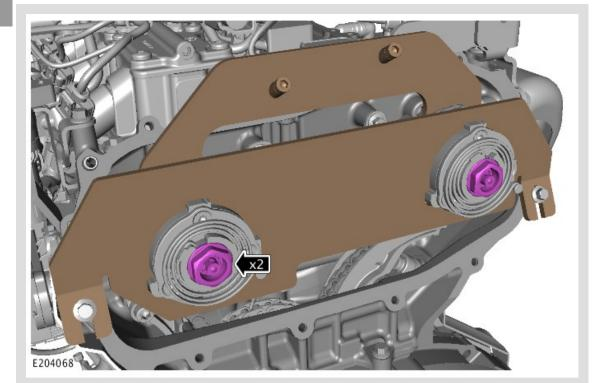
• Loosen, but do not fully remove the Variable Camshaft Timing (VCT) bolts.
