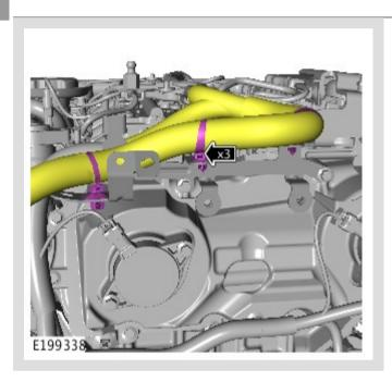
Remove the 3 clips and release the upper wiring harness from the support bracket.
