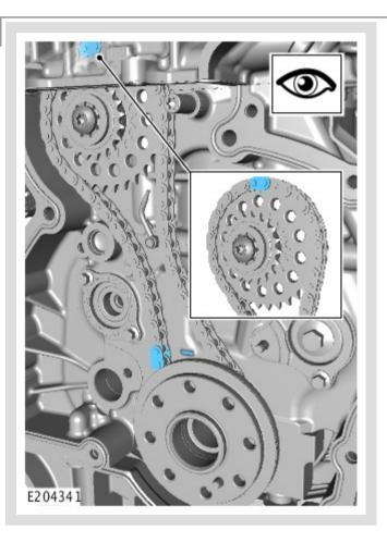
Make sure that the timing marks are aligned as illustrated
