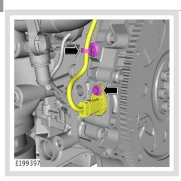
Remove the crankshaft position (CKP) sensor.
