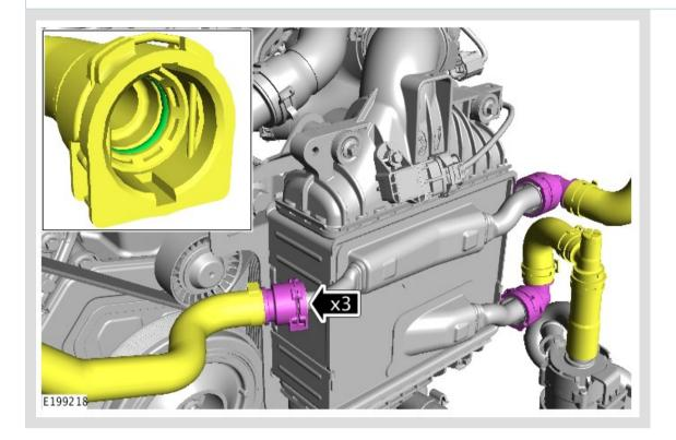
Disconnect the 3 engine coolant hoses from the charge air cooler.
