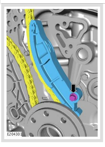
Remove the timing chain tensioner guide and bolt.
