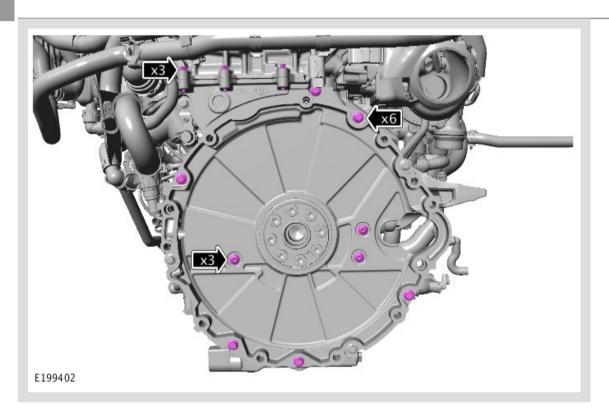
Install the remaining 12 bolts and tighten to the correct torque.
