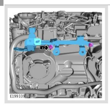
Remove the upper wiring harness support bracket.
