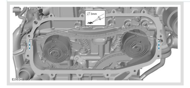
Apply a 3mm diameter bead of RTV sealant to the upper timing chain cover gasket in the position shown. Refer to: Specifications (303-01 Engine - INGENIUM I4 2.0L Petrol, Specifications). *Renew Part: Timing chain cover gasket Quantity: 1 .*
