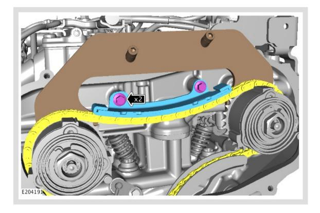
Install a new upper timing chain guide.
