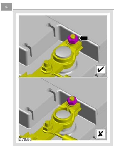
Make sure the battery monitoring system (BMS) electrical connector is connected to the module, before installing the BMS on to the battery terminal.
