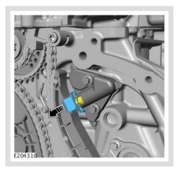
Release the lower timing chain tensioner piston.
