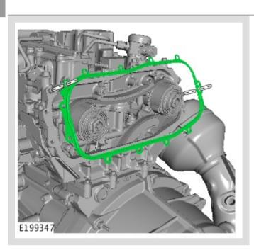
Install the upper timing chain cover gasket.
