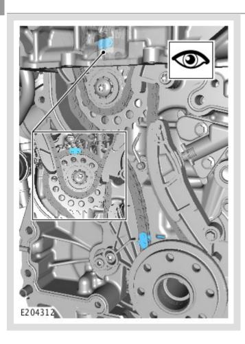
Make sure that the timing marks aligns as illustrated.
