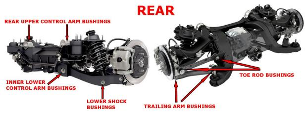
18. Once all the bushings are loose, bounce the car a few times to re-index the bushings then tighten using the following chart:
