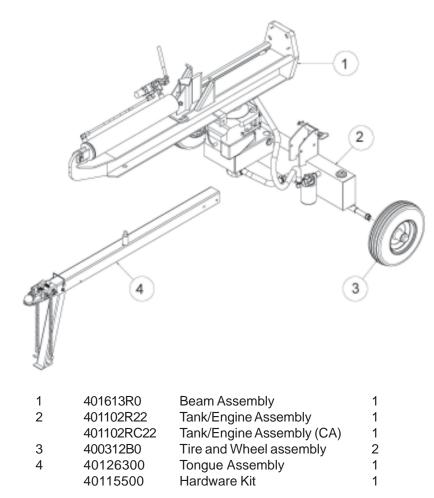
**NOTE:** This log splitter was partially assembled at the factory. Refer to the drawing and parts list should it become necessary to disassemble the unit for repair or replacement of parts.
