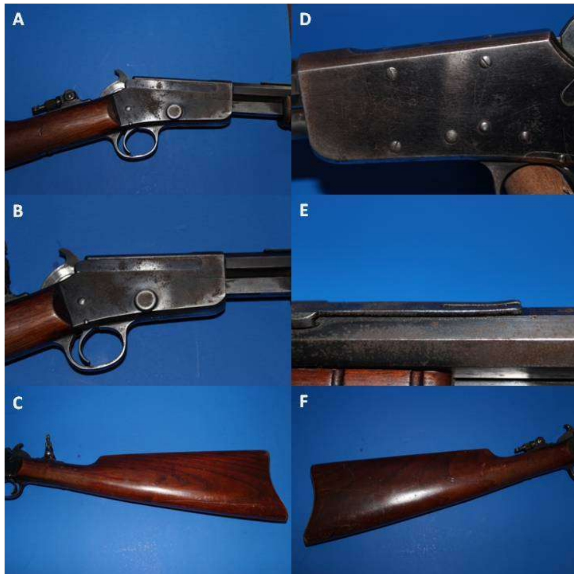
BEFORE RESTORATION The pitting on the right side of the receiver can be observed in panels A and B. "P.F. Coe 1907" has been scratched into the left side of the receiver (panel D). Note the dents and scratches in the stock in panels C and F. The barrel mounted sight is missing its slider (panel E).
