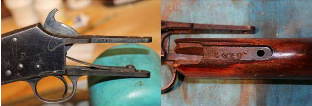
The serial number is located on the left side of the upper tang. The stock must be removed to read the serial number (clearly, the Model 20 was made before the BATFE was formed). Note that the
