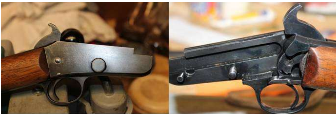
The rear portion of the receiver is shown following bluing with Oxpho-Blue. Note that the deep pitting seen in the "BEFORE" pictures is lacking. The simplicity of the trigger is shown in the right picture. Even though the trigger mechanism is simple, the trigger pull is exceptionally smooth, light, and crisp.
