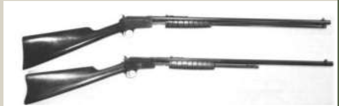
A Model 20A with a full length magazine is shown in the top picture, along with a Model 20 with a half length magazine.
