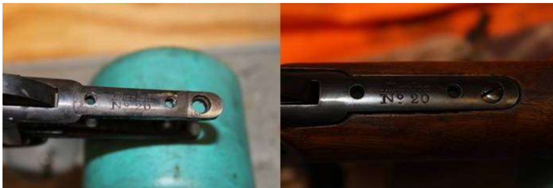
The top tang before bluing showing "Marlin No. 20." the tang rear sight must be removed to see the model number. On the right, the deep blue is shown after application of Oxpho-Blue.
