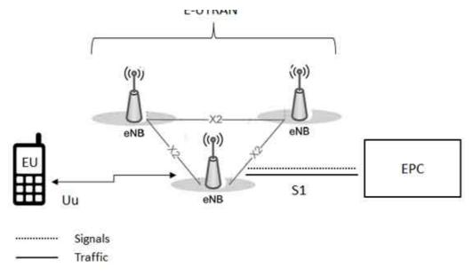
The E-UTRAN handles the radio communications between the mobile and the evolved packet core and just has one component, the evolved base stations, called **eNodeB** or **eNB**. Each eNB is a base station that controls the mobiles in one or more cells. The base station that is communicating with a mobile is known as its serving eNB.
