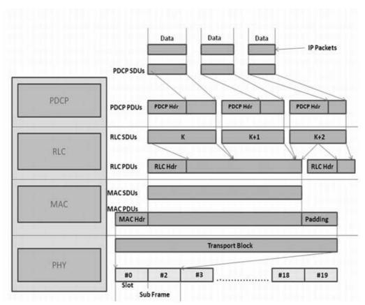
Packets received by a layer are called Service Data Unit SDU while the packet output of a layer is referred to by Protocol Data Unit PDU. Let's see the flow of data from top to bottom:
