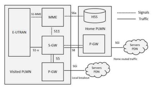
The home network's P-GW allows the user to access the home operator's services even while in a visited network. A P-GW in the visited network allows a "local breakout" to the Internet in the visited network.
