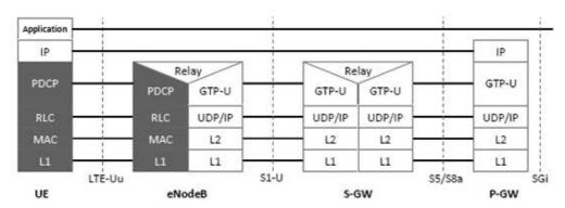
Packets received by a layer are called Service Data Unit SDU while the packet output of a layer is referred to by Protocol Data Unit PDU and IP packets at user plane flow from top to bottom layers.
