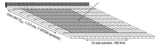
Each user is allocated a number of so-called resource blocks in the time.frequency grid. The more resource blocks a user gets, and the higher the modulation used in the resource elements, the higher the bit-rate. Which resource blocks and how many the user gets at a given point in time depend on advanced scheduling mechanisms in the frequency and time dimensions.
