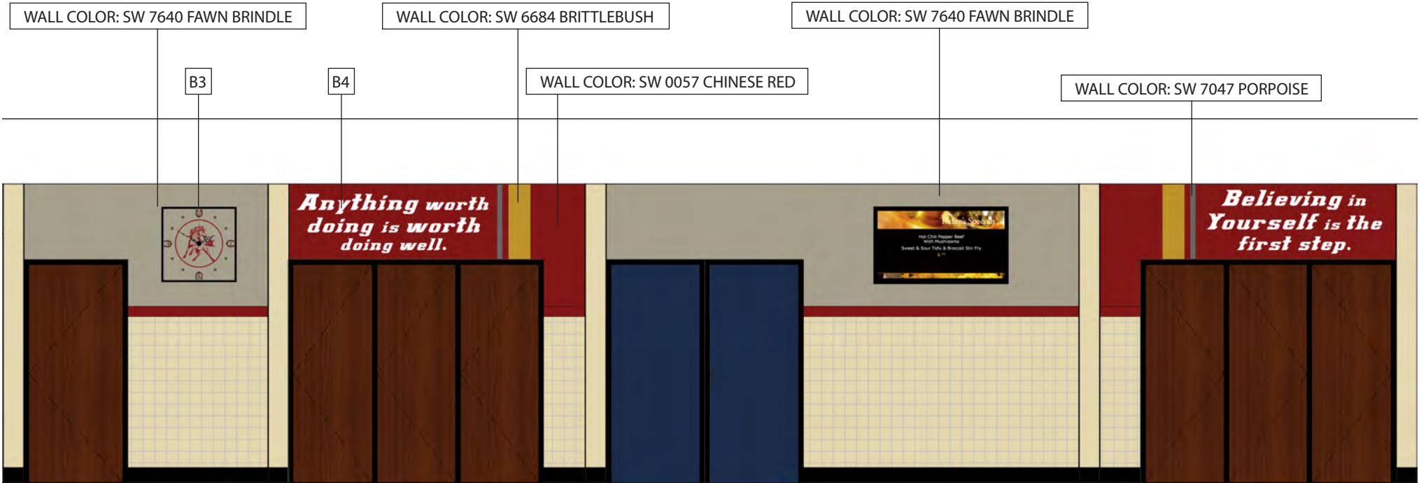
B3: Custom Mustang Clock B4: Vinyl Graphic Applied to the Second Surface
