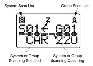
The type of scanning selected is determined by the menu mode SCN TYPE parameter (see page 32). If that parameter is not selectable, the type of scanning is fixed by programming. The available scan types are as follows.
