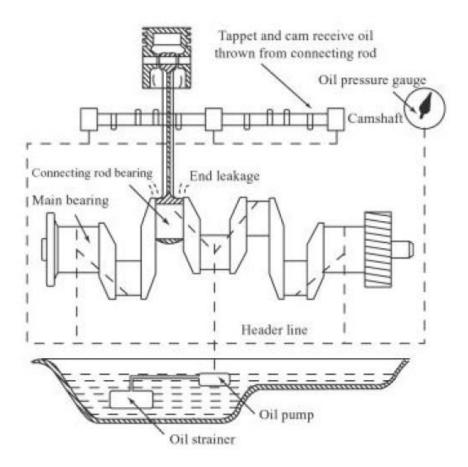
This system provides sufficient lubrication to all parts and is favoured by most of the engine manufacturers. This is used in most heavy duty and high-speed engines.
