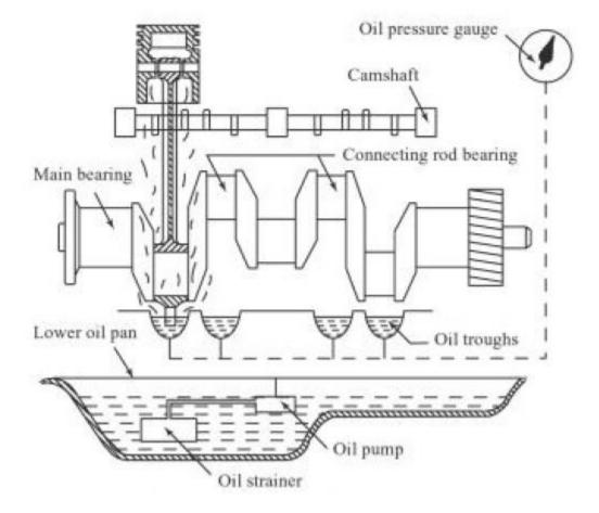
A hole is drilled through the connecting rod cap through which the oil passes to the bearing surface. Oil pockets are provided to catch the splashed oil over all the main bearings and also the cam shaft bearings. From these pockets oil passes to the bearings through drilled hole. The surplus oil dripping from the cylinder flows back to the oil sump in the crank case.
