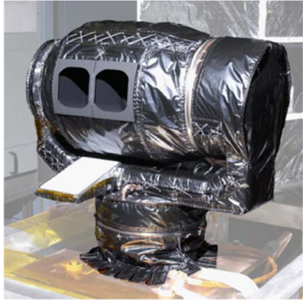
Fig. 6 The MRO MCS flight model during thermal vacuum testing at JPL
