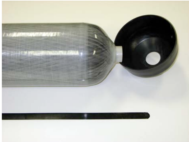
Photo 2: Cylinder surface after cap has been removed.
