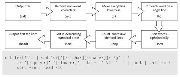
Each command does one simple thing: cat reads a file from disk; sed edits the file; tr changes one set of characters to another; sort sorts the data; uniq removes duplicates from sorted data and counts occurrences; and head outputs the first several lines of its input. Connected in the proper order, they perform a far more complex task: list the ten most common words in a text file.
