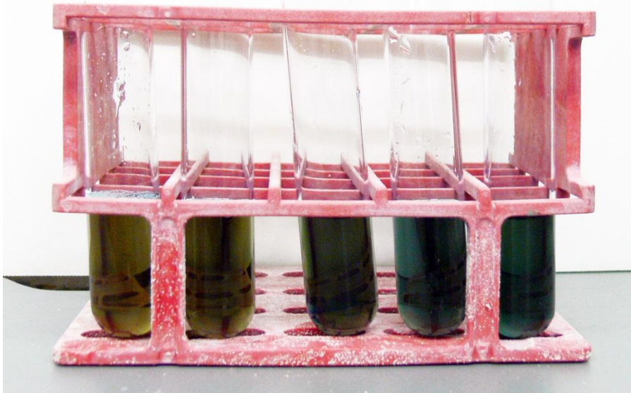
Figure 12. This figure shows the effect of the BSA protein on the absorbance of the Bradford reagent. The left test tube has zero protein added, and appears light brown. Each test tube from left to right increases in BSA protein by 10 \mu\text{l} . The far right test tube contains 40 \mu\text{l} of BSA protein, and appears dark blue. The absorbance of each test tube will be used to create the standard curve.
