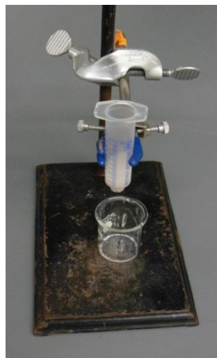
Figure 10. Syringe column with removed pressure pump and glass wool and hydrated Sephadex.
