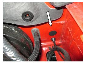
STEP 6: Remove breather hose by depressing safety clip and sliding the tube off of the intake tube.
