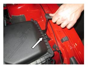
**STEP 10:** Remove 2 screws from the mass airflow sensor and remove from the production intake tube.
