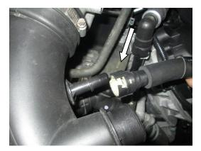
STEP 7: Loosen both intake tube hose clamps at the throttle body and air-box assembly.
