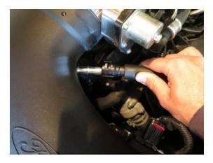
STEP 19: Connect the mass airflow meter connector, ensuring the safety clip is in the locked position.
