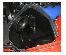
STEP 17: Install the intake tube onto the throttle body with 1 large hose clamp then over the air filter adapter with 1 medium hose clamp. Torque all clamps to 44.25 in-lb +/- 1.75 in-lb (5.0 Nm +/- 0.2 Nm).
