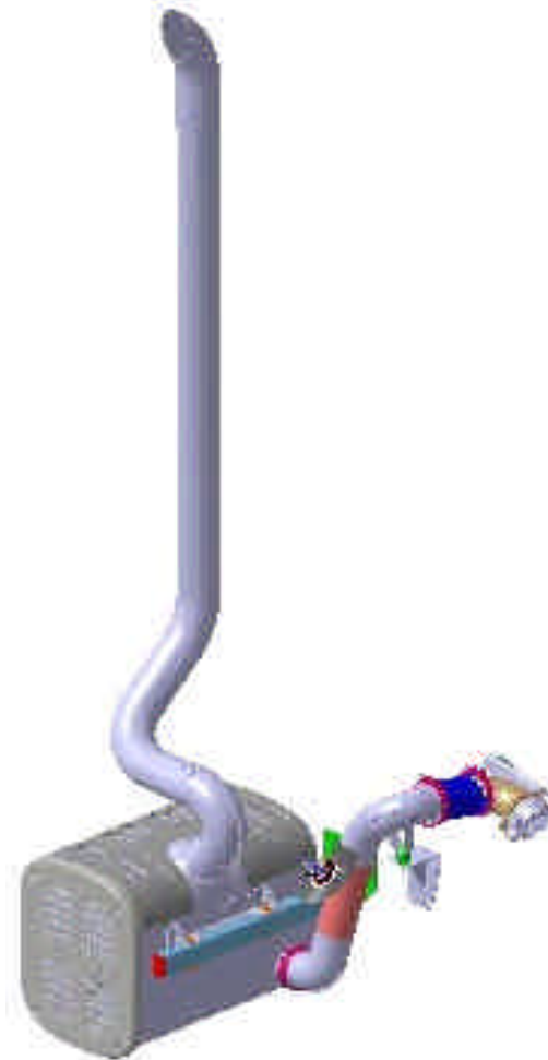
VERTICAL EXHAUST PIPE (CCP 180)
