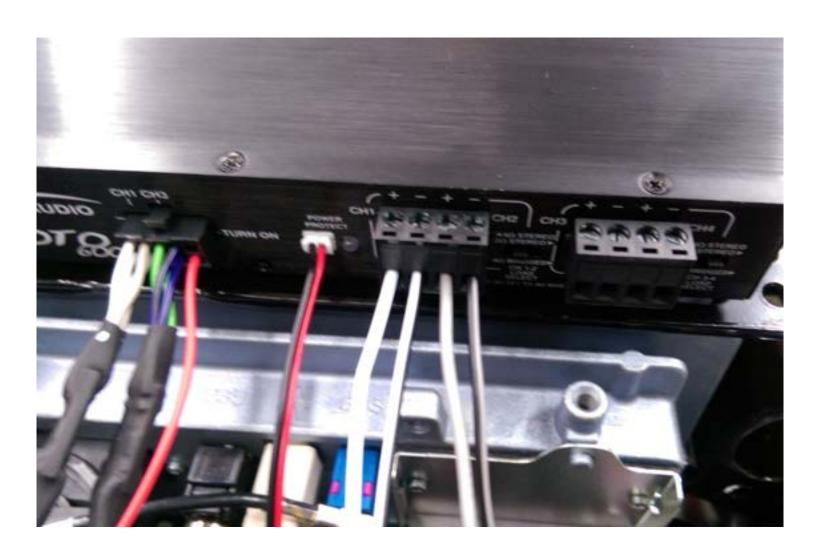
27. On the end of the speaker harness are 4 stripped wires. Connect them to the 4 screw block terminal on the end of the amplifier with the controls.
