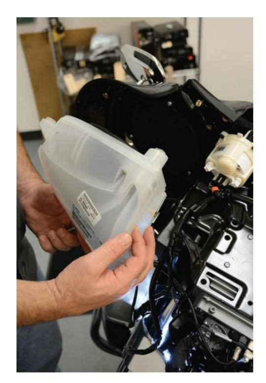
The enclosure should be loose and come off freely. If the enclosure does not come off easily don't force it, repeat these steps and insure you have fully removed all fasteners.
