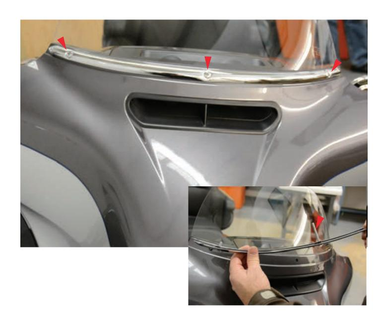
11. Remove the 3- Philips head screws below the windshield. Warning: The outer faring is loose and ready to remove. Don't let it fall. It maybe helpful to leave the center (long) screw in place and loose until you are ready to remove the fairing and windshield.
