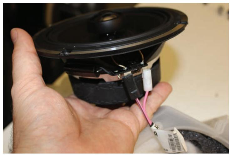
20. Plug in the new speakers using the original factory connectors. Note: There are 2 sizes of connector. Use the larger, black connector on the larger speaker terminal regardless of the wire color. We have compensated for this elsewhere in the wiring harness.
