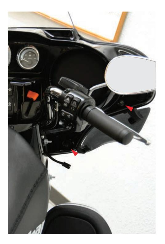
10. Remove the 4- T25 Torx head screws at the inside edge of the inner fairing. Note: it maybe necessary to remove the fog lights it equipped.
