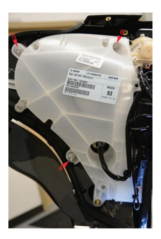
17. Remove 3-3/16" Allen head screws (4, 5 and 6). Nothing special here. You may find a small magnet useful for removing screw 6.
