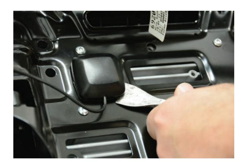
22. You will need to relocate this antenna module if it is equipped with GPS. It is attached with double stick tape. Pop it off and move it up on the bracket to the right.
