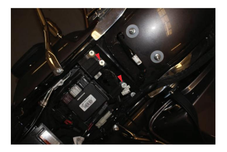
8. Remove the 2 highlighted bolts. You may find it helpful to remove the control module (the one with 3 big plugs on it) on top of the battery cover.
