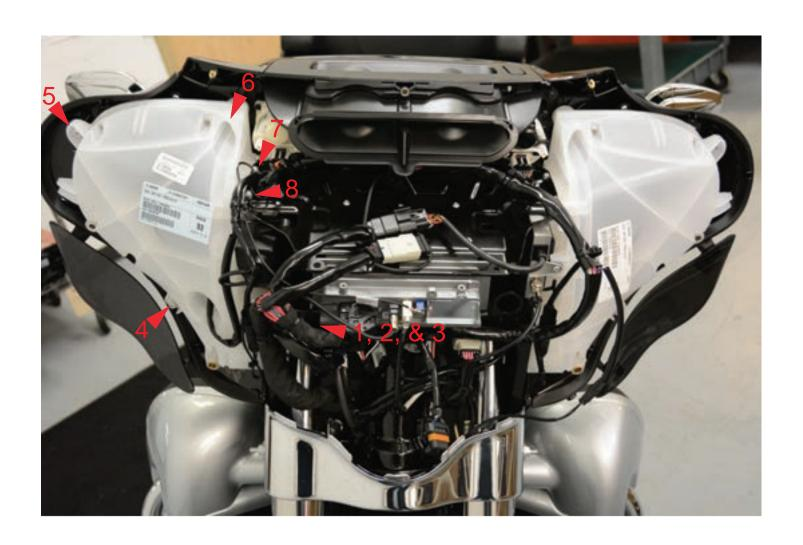
13. This is what you should see when you outer fairing is removed. To access the speakers you will need to remove the 8 fasteners that secure the speaker enclosures to the inner fairing. Note: These enclosures are a structural part of the fairing. All the fasteners must be use and tight when reinstalling the speaker enclosures.
