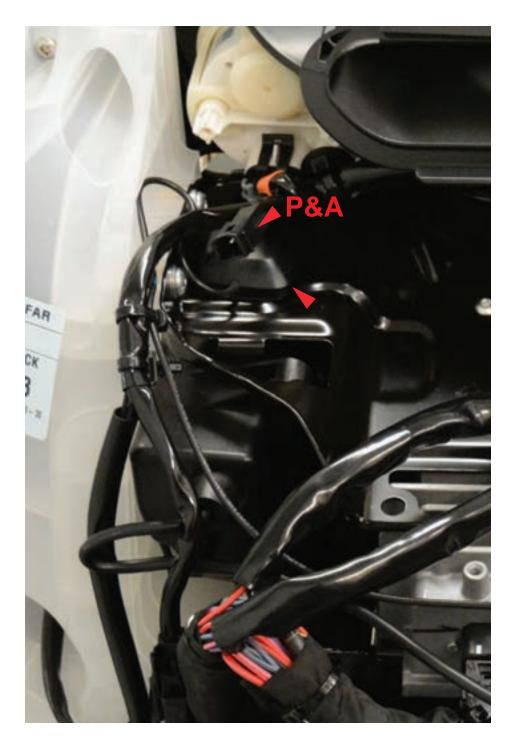
23. This also happens to be the approximant location of the wire we will use for remote turn on. The service manual calls this a "P&A" connector and it is intended to power or trigger accessories like this. There will be an empty plug in the end that will need to be removed. Once that cap has been removed you can plug in the provided orange wire and set it aside.
