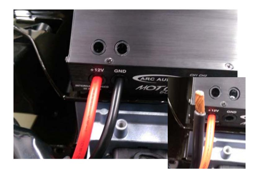
25. Connect the power harness from the battery to the 3 screw terminal block on the end of the amplifier. You did remember to remove the fuse from the harness right? The Red wire goes to the +12V terminal, black to GND and the orange wire from the P&A connects to TURN ON.
