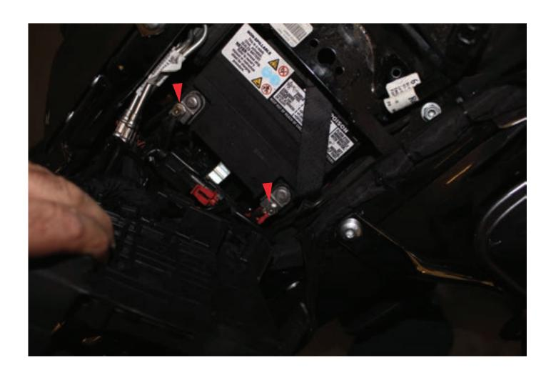
9. You have now exposed the top of the battery. The 2 ends of the power harness with the metal ring terminal can now be connected to the battery at this location. Take extra care when working around the positive (+) battery terminal. You should always wear safety glasses when working with the battery.
