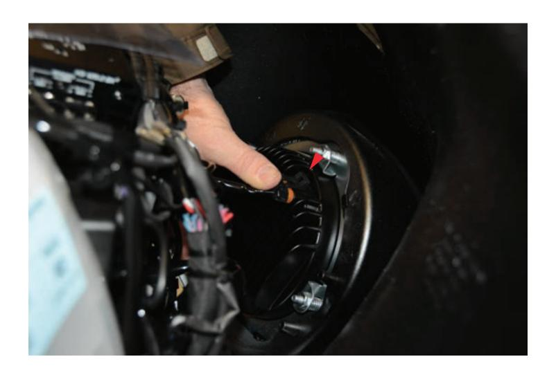
12. Gently pull the outer fair toward you. You will need to lean over the fairing and locate the headlight wiring harness. Disconnect the headlight harness and let it hang. If no aftermarket accessories have been added, you can now remove the fairing. Set it is a safe, out of the way location where it will not be dropped or damaged
