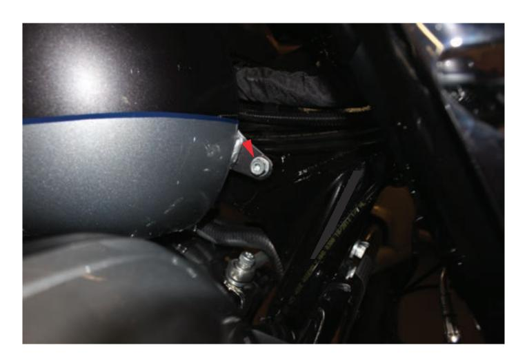
3. Remove the 2 bolts at the front of the tank. These are under rubber covers that must be removed first.
