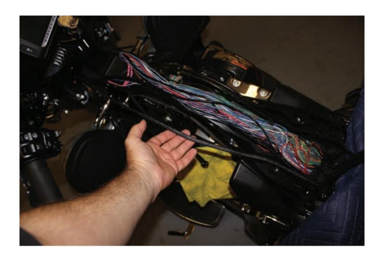
6. Remove the black plastic cover off the top of the wire cover on the back bone of the frame. No tools here, just work it loose from the tabs.
