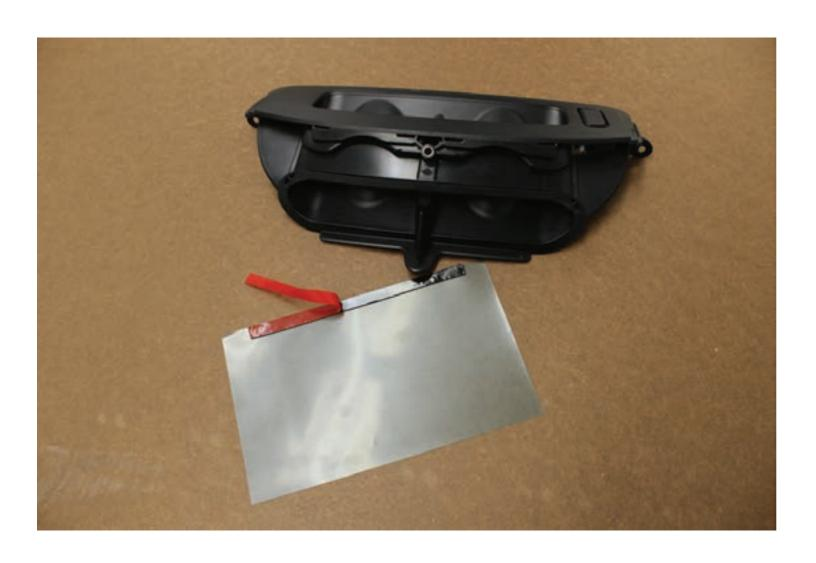
28. Apply the protector to the bottom side of the vent assembly. Clean the surface with alcohol and allow it to dry thoroughly. Peel the protective strip from the double sited tape and stick it to the bottom of the vent assembly making sure it is approximately centered.
