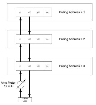
Figure 5: Wiring Meters in Parallel
