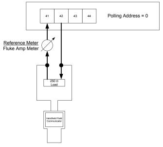
Figure 6: Setup to Assist in Calibrating Analog Output
