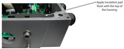
Figure 4: Installing Foam Insulation Pad
