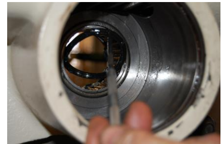
REPLACE HOUSING SEAL- BLACK LIP FACES BEARING!
