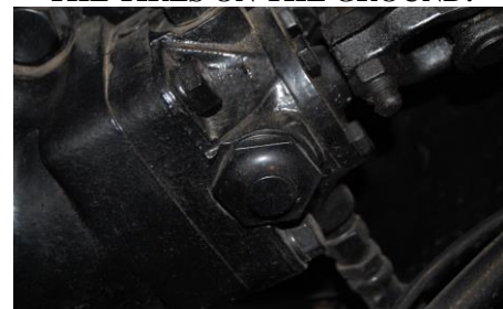
PRV IN BEARING CAP
