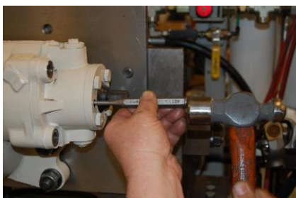
RESET BOTH AUTO PLUNGERS IF THE O-RINGS WERE REPLACED
