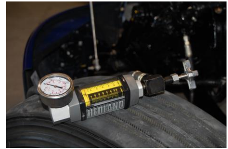
PRESSURE & FLOW TESTER
