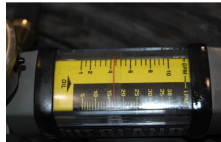
FLOW W/ 1500 PSI LOAD APPLIED
