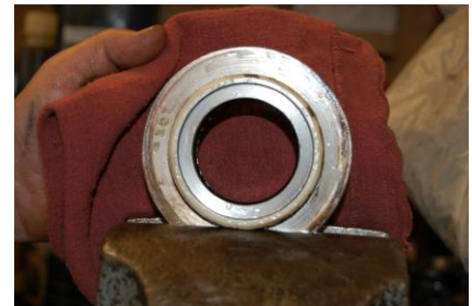
SEALS MUST BE PERFECTLY ROUND-NO FLAT SPOTS!!
