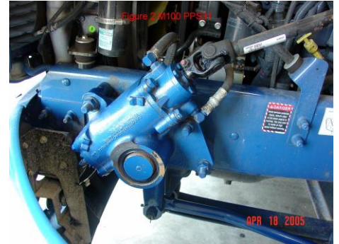
SELF-BLEEDING GEAR (SECTOR BORE IS BELOW CYLINDER)
