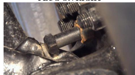
AXLE STOP W/ TYPICAL GAP
