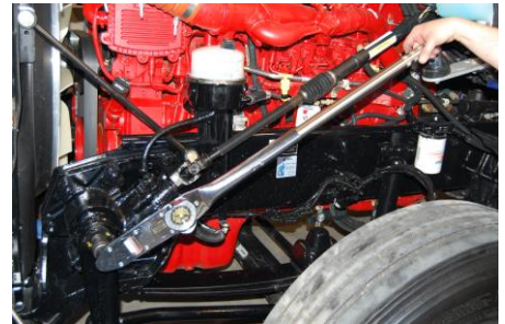
TORQUE THE RETAINER
