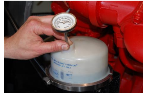
PERFORM TESTS AT 180F
