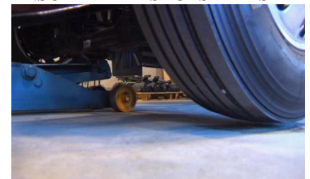
JACK UP STEER AXLE AND TURN FROM STOP TO STOP
