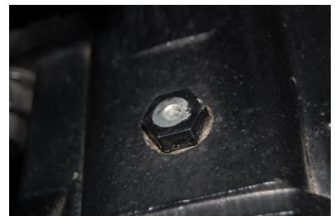
BLEEDER PLUG (WITH TAPE REMOVED). BLEED ONLY WHEN TURNING RIGHT!
