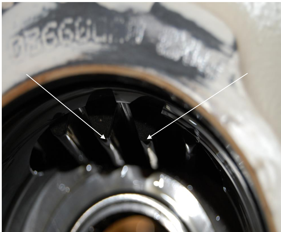
TIMING MARKS ON THE 2 CENTER TEETH OF THE PISTON RACK
