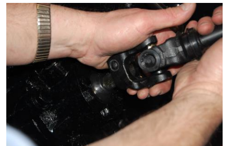
CHECK U-JOINTS AND SLIDER
