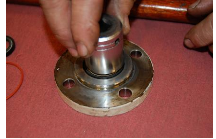
INPUT SEAL GOLD SPRING FACES OUT!
