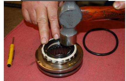
TAP IN NEW EXCLUDER AND REPLACE O-RING
