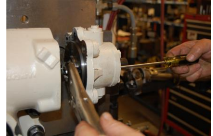
REPLACE THE AUTO PLUNGER O-RING IF NECESSARY
