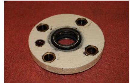
SALT SEAL SILVER SPRING FACES OUT!
