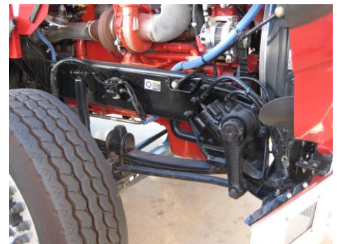
DUAL GEAR SYSTEM SLAVE GEAR
