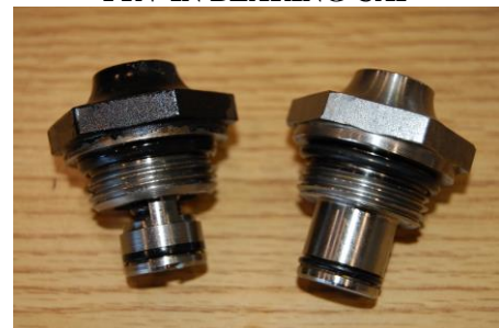
PRV ON LEFT, 3331812K TEST PLUG ON RIGHT
