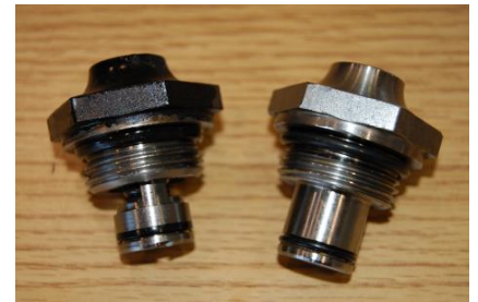
LEFT-PRV, RIGHT 3331812K TEST PLUG
