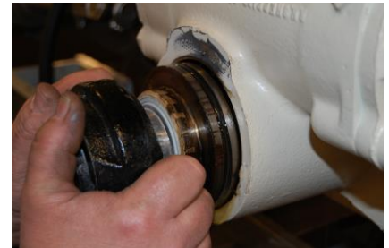
PITMAN ARM USED AS A HANDLE TO PULL SHAFT
