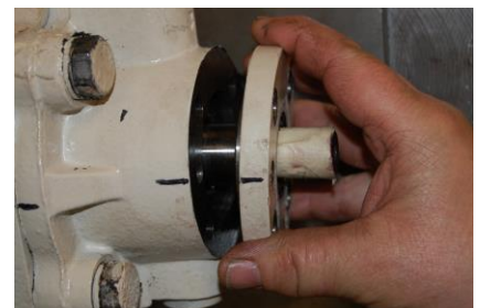
INSTALL COVER AND TORQUE THE BOLTS TO 53-64 FT
