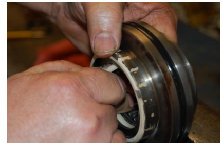
INSTALL NEW SEAL-BLACK LIP FACES THE BEARING!
