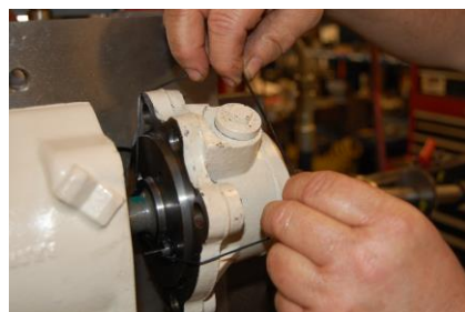
STRETCH NEW SQUARE RING OVER THE BEARING CAP
