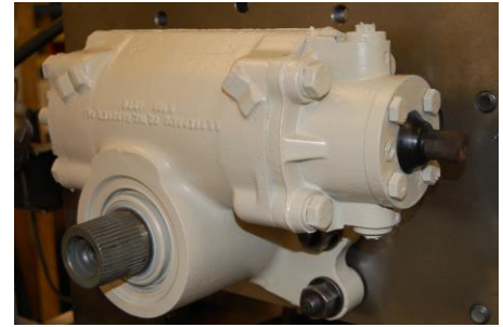
PITMAN ARM AND COLUMN REMOVED
