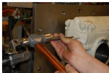
RESET BOTH AUTO PLUNGERS IF THE O-RINGS WERE REPLACED
