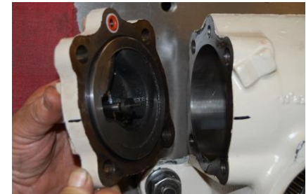
INSTALL AND TORQUE BOLTS
