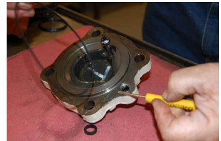
REPLACE THE SEALS
