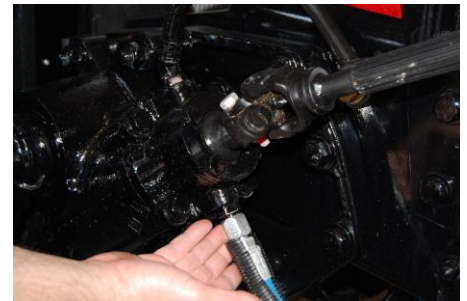
INSPECT FOR LEAKS AND KINKS
