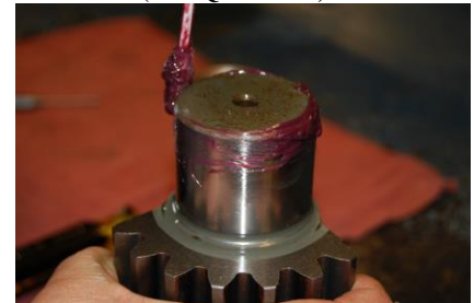
GREASE THE SHAFT!
