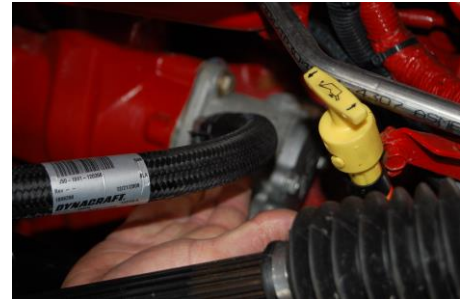
INSPECT THE LINES FOR KINKS
