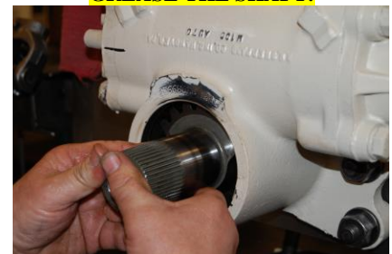
ALIGN THE TIMING MARKS!
