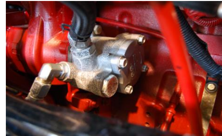
TYPICAL STEERING PUMP
