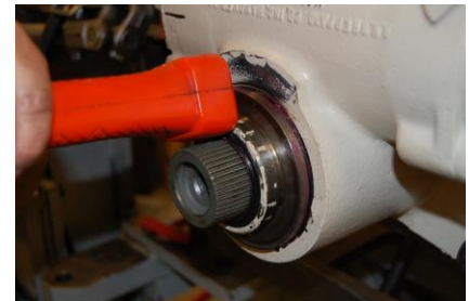
INSTALL THE COVER AND SNAP RING (OR CLIPS & BOLTS)
