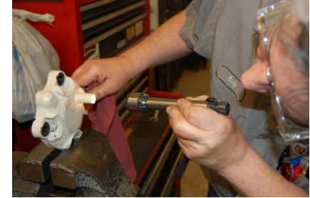
INSPECT AND CLEAN BORE
