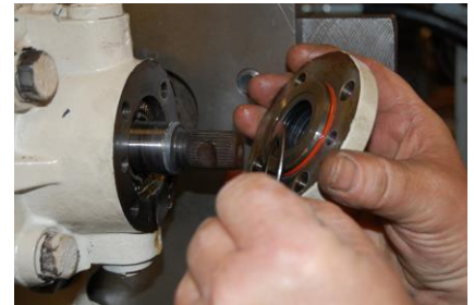
REMOVE COVER AND REINSTALL SHIM
