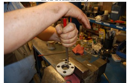
DRIVE THE INPUT SEAL OUT
