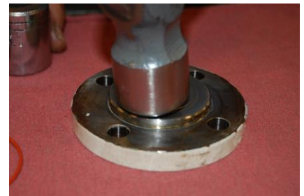
REINSTALL COVER WASHER AND O-RING
