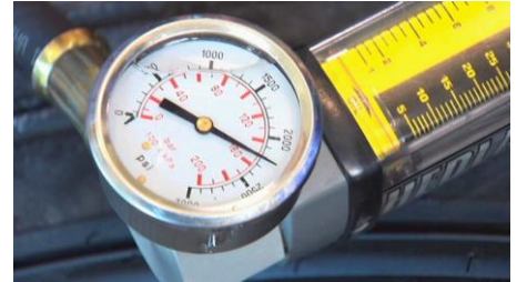
MAX PUMP PRESSURE AND NO FLOW = 0 INTERNAL LEAKAGE
