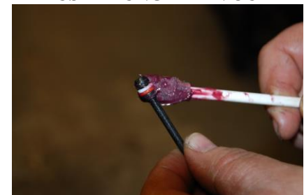
GREASE THE NEW O-RING!
