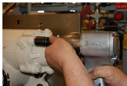
REMOVE BEARING CAP BOLTS
