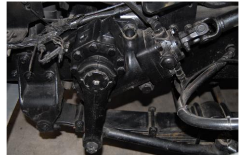
GEAR WITH BLEEDER (SECTOR BORE IS ABOVE CYLINDER)
