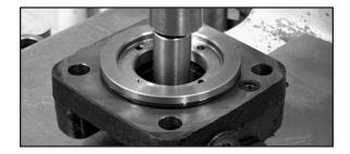
10. Press the salt seal into the bearing cap until it is flush with the face of the cap. Coat both seals with clean grease before installing the rotary valve shaft.
