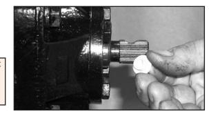
4. Separate the bearing cap assembly from the housing by turning the input shaft out of the housing. Turn the shaft until it stops.
