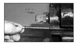
**IMPORTANT**: If your steering gear was originally built with a grease fitting in the bearing cap, remove the fitting and fill the hole with RTV to prevent ingestion of contaminants. No further lubrication is required.
