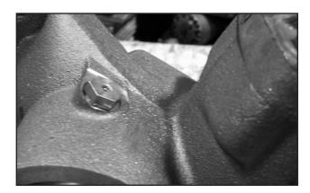
7. Locate the bleeder screw in the plug located on the sector shaft bore (Figure 34).
