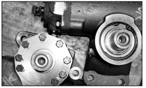
Clean the shaft and remove the sector shaft cover. It may be necessary to crank the engine to force the cover out of the housing
