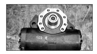
Disassembled Slave Steering Gear - M-Series.
