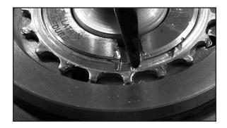
17. Install a new O-ring and tetra-seal in the bearing cap. Coat both seals with clean grease for installation. Install the boot over the input shaft splines.
