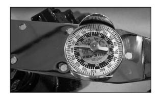
4. Continue torquing the retainer past the specified value until two of the notches in the retainer align with the tabs of the washer.
