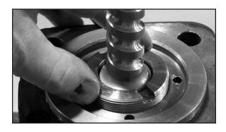
**NOTE**: Valve pre-load can be measured by turning the input shaft with an inch pound torque wrench. When properly set the radial drag will not exceed 25 inch pounds.
