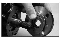
WARNING DO NOT TURN THE INPUT SHAFT DURING REPAIRS. DAMAGE TO THE STEERING GEAR WILL RESULT.
