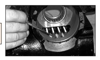
14. Align the marks on the bearing cap with the marks on the housing. Install the four attaching bolts in the bearing cap assembly and torque to specifications.
