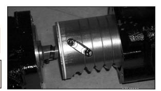
10. Hold the shaft assembly stationary and install both halves of the ball return tube. Continue feeding the balls through the access hole in the ball return tubes until 24 balls have been installed.
