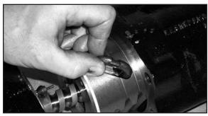
14. Carefully turn the shaft to remove the re-circulating balls from the piston. All M-Series steering gears will have 24 balls. Verify that all balls are removed before removing the valve shaft from the piston.
