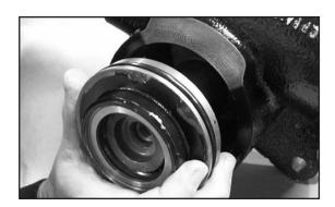
11. Install the snap ring or attaching bolts in the cover.
