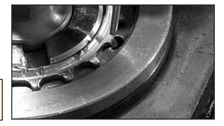
**CAUTION** Do not bend the locking tabs into the threaded plunger hole in the bearing cap.
