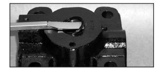
8. Using an appropriate size seal driver, push the oil seal out of the bearing cap.
