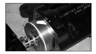
13. Slide the piston into the housing until the rack gear is centered in the sector shaft bore of the housing. Locate the timing marks on the piston rack for reference.
