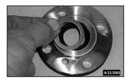
2. Install the protective washer (if equipped) into the bearing cap cover using an arbor press and suitable size seal driver. Install a new o-ring on the bearing cap cover.
