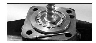
2. Use the chisel and hammer to split the star nut at the grooves of the adjusting nut. Remove and discard the star nut.
