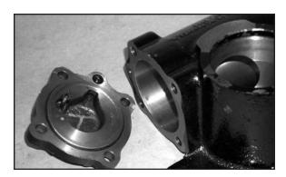
19. Remove the sector shaft oil seal from the housing.
