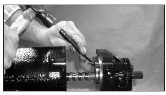
9. With the flange against the spring pin, use the center punch to stake the threads of the plunger body Take care to not bend the plunger when staking the threads.
