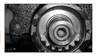
16. Install a new sector shaft oil seal in the sector shaft cover. When properly fitted the seal will ride between the roller bearing and cover. The black lip of the seal must face the bearing.
