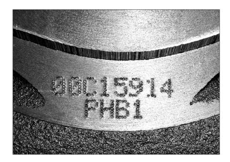
A number is cast into the steering gear housing and identifies the basic family the steering gear belongs to.
