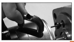
11. Replace the O-ring on the ball guide retainer and install the ball guide retainer over the ball return tubes.
