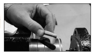
12. Slide the piston into the housing until the ball guide retainer is secured by the housing. Locate the rack gear of the piston with the opening in the housing at this point.
