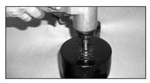
2. Remove all external seals from the steering gear, including the sector shaft dust boot, snap ring protective cover (if equipped), frame side protective disk and the input shaft dust boot.
