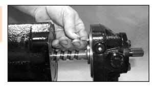
6. Coat the O-ring of the plunger assembly with a light coat of grease and install the plunger body through the spring pin.
