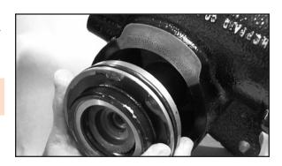
or below the groove in the housing. Improper installation can result in separation of the cover without warning. Personal injury or an accident can result.
