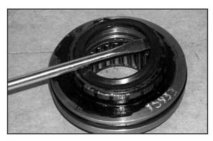
9. Remove the four attaching bolts from the bearing cap and turn the input shaft to free the bearing cap assembly from the housing. Turn the shaft until the plunger clears the piston.
