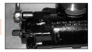
15. Install the sector shaft by carefully aligning the timing mark of the sector shaft with the two timing marks of the rack piston. It will be necessary to tap the sector shaft into place with a soft hammer to ensure full rack engagement.
