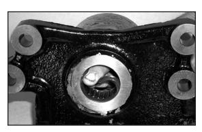
9. Install the sector shaft into the housing taking care to align the timing mark on the sector with the timing marks on the piston. It may be necessary to tap on the sector shaft to properly seat it into the housing.
