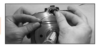
6. Insert the valve shaft into the ball thread of the piston.
