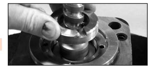
5. Remove the inner thrust assembly from the valve shaft. Note the order of the thrust assembly for reassembly.
