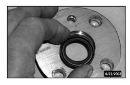
3. Press the salt seal into the cover until it is flush with the face of the cover. There is a choice of two salt seals for the M-series gear. Select the proper salt seal for your cover and press it into the cover until it is flush with face of the cover.
