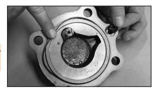
19. Replace the O-rings on manually adjustable plungers and install them into the end caps.
