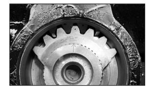
10. Install the sector shaft cover onto the steering gear. Insure that the cover is properly seated when installing. Snap ring covers must be flush or below the snap ring groove when properly installed.
