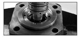
6. Remove the outer thrust assembly from the bearing cap bore. Note the order of assembly for reassembly.
