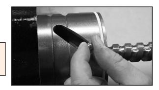
8. Slowly turn the input shaft into the piston while feeding the balls into the ball guide feed hole. As you feed the balls you will feel the shaft being supported as the balls fill the threads.
