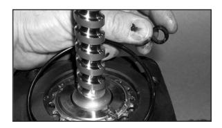
18. Install the plunger into the bearing cap. Reassemble the steering gear following the procedures in the re-assembly portion of this manual.
