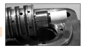
12. Carefully install the rotary valve shaft into the bearing cap. Do not damage the input shaft oil seal when installing the valve assembly. Do not turn the shaft during installation. Remove the tape from the splines.
