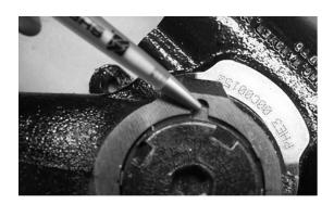
**IMPORTANT**: Take note of the torque <u>value on the face</u> <u>of the retainer</u>. Always torque the retainer to the specified value.
