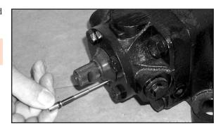
20. Install the excluder seal in the sector shaft cover using a 2.25" seal driver. Pack the lip of the excluder seal with clean chassis grease before installing. When properly installed the lip of the excluder will face outward and the seal will bottom in the excluder seal groove.
