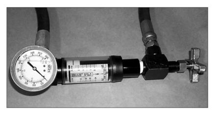
This tester is a self contained, direct reading device to check system flow, pressure or both at the same time. It can detect worn components, check flow and pressure control settings or monitor overall system performance.
