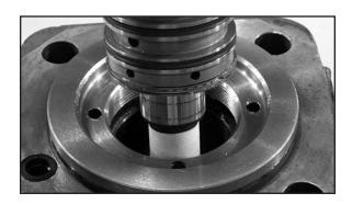
13. Install the inner thrust assembly onto the rotary valve shaft. The thrust bearing will ride on the face of the valve and the thrust washer will ride against the shaft retaining nut.
