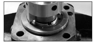
4. Carefully remove the valve shaft from the bearing cap. Do not turn the shaft during removal as seal damage could result.
