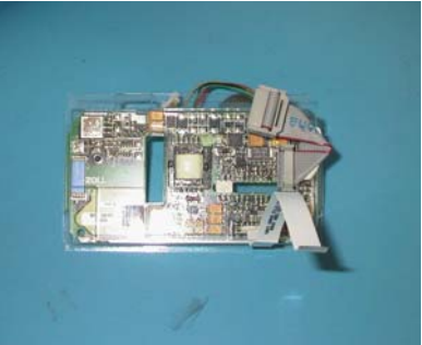
Isolated Power Supply for SpO 2 Module
