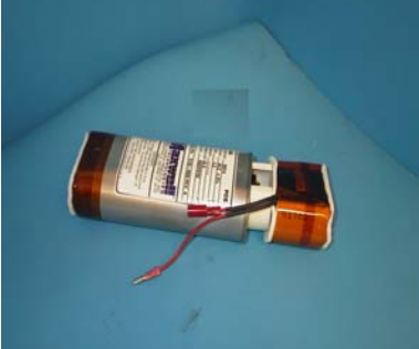
High Voltage Capacitor Assembly
