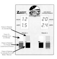
buttons also perform secondary functions (shown in white letters with blue background) when the Z-4000 is in Program mode. For more information on using the buttons, see the "Basic Operating Instructions" and "Programming Proto-Sound® Features" sections of these operating instructions.
