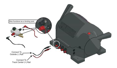
Once the track and/or accessories have been wired up to the Z-4000, plug the AC power cord into any 110V household plug and follow the remaining operating instructions.
