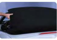
**3** Fold back top and push firmly on front of top to securely lock in open position.
