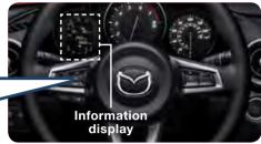
Push and hold the center of the INFO button to reset the currently displayed feature such as Average MPH or Average MPG.
