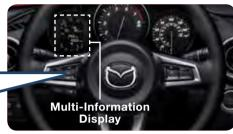
Push and hold the center of the INFO button to reset the currently displayed feature such as Average MPG.
