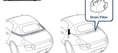
**NOTE:** Manual Convertible Top Maintenance: Remove leaves or other matter that may accumulate around the area where the soft top meets the vehicle body to prevent water drainage filters from becoming clogged. Clogged water drainage filters may result in water intrusion into the passenger compartment. For detailed maintenance of the water drainage filters, refer to MyMazda.com or consult an Authorized Mazda Dealer.
