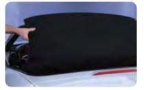
If closing from outside vehicle, grasp side of top near windshield header.
