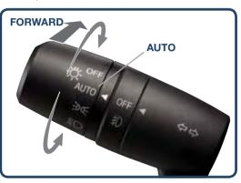
When the HBC system is on, the HBC indicator light in the instrument cluster will illuminate (AMBER). The High Beam indicator light will turn on (BLUE) when the HBC system switches to high beam and will turn off when the HBC system switches to low beam.
