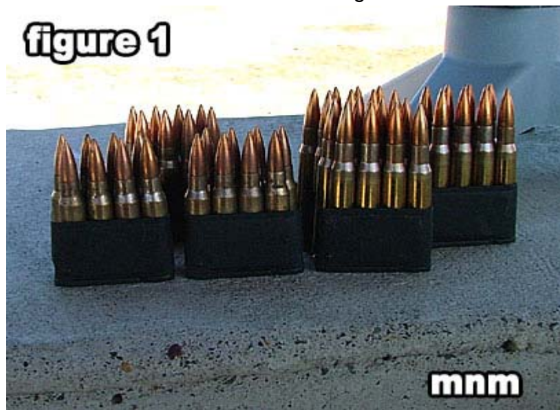
7.62x51 NATO loaded enbloc magazines sitting to the left of 30-06 cartridges in enbloc magazines.
