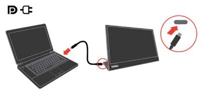
2) Connect the USB-C port of mobile phone and M14 with a USB type-C cable. (Electronically marked cable, current rating: 5A)
