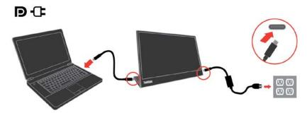
Connect Type-C power adapter to the left or right side of M14 and connect M14 to the mobile phone with a USB-C cable. (Electronically marked cable, current rating: 5A)
