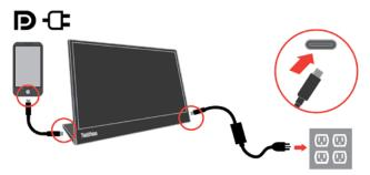
NOTE: When you encounter abnormal charging condition, please check your power capacity of power adapter connected with M14 and make sure it is enough for M14 and other devices.
